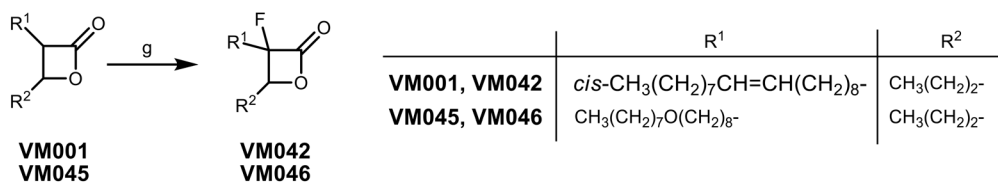
Scheme 3 Synthesis of fluorinated \beta -lactones (methods C & D). Reagents and conditions: (a) i) CDI, dry THF, r.t., 6 h; ii) MgCl 2 , EtOCOCH 2 COOK, r.t., 18 h; iii) aq. HCl 1 N, 95%; (b) K 2 CO 3 , R 1 , acetone/DMF, reflux, 18 h, 67–70%; (c) i) NaH, dry THF, –20 °C, 1 h, ii) Selectfluor, dry MeCN, –20 °C, 2.5 h, 78–82%; (d) NaBH 4 , EtOH, 0 °C 30 min, then r.t. 3 h, 61–82%; (e) NaOH 1 N or LiOH 1 N, THF or 1,4-dioxane, r.t., 16 h, 51–75%; (f) EDC·HCl, DMAP, dry DCM, r.t., 72 h, 29–36%; (g) i) LDA (prepared in situ from (i-Pr) 2 NH and n -BuLi), dry THF, –78 °C, 30 min, ii) NFSI, dry THF, –78 °C to r.t., 2.5 h, 23–39%.
