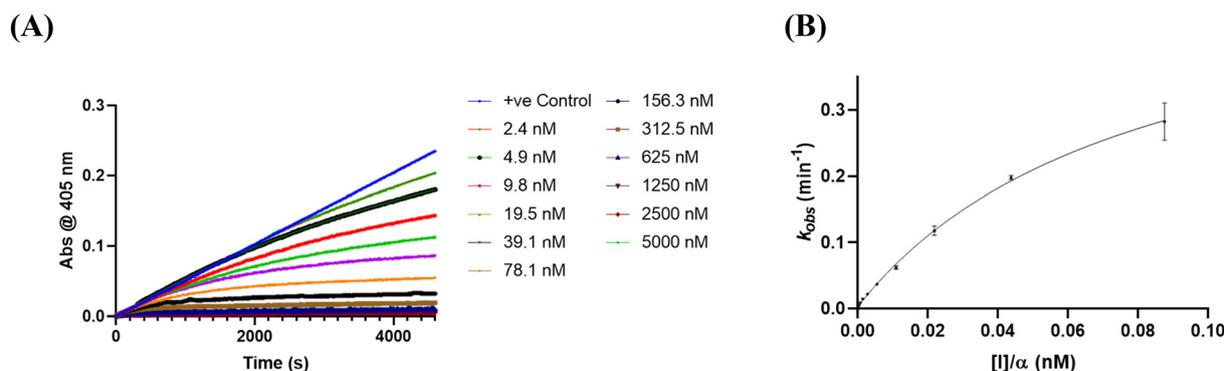
**Fig. 4** Continuous activity assay with saxagliptin, DPPiV, and Gly-Pro-pNA. (A)  $k_{\text{obs}}$  values were fitted from reaction progress curves of absorbance vs. time at different concentrations of saxagliptin using eqn (S12). (B) Saturation fitting of these  $k_{\text{obs}}$  values according to eqn (4) provided values for  $k_5$ ,  $k_6$ , and  $K_i$ .
