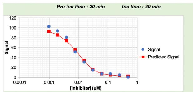
Fig. 8 Global fitting of pre-incubation time dependent  $IC_{50}$  datasets obtained for saxagliptin, using EPIC-CoRe.  $IC_{50}$  curves were obtained for pre-incubation times ranging from 0–20 min and incubation times fixed at 20 min.
