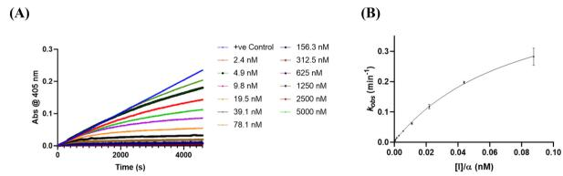
Fig. 4 Continuous activity assay with saxagliptin, DPPIV, and Gly-Pro-pNA. (A)  $k_{\rm obs}$  values were fitted from reaction progress curves of absorbance vs. time at different concentrations of saxagliptin using eqn (S12). (B) Saturation fitting of these  $k_{\rm obs}$  values according to eqn (4) provided values for  $k_5$ ,  $k_6$ , and  $K_i$ .
