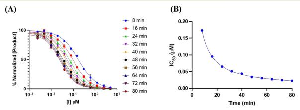
Fig. 6 Incubation time-dependent IC<sub>50</sub> experiment with saxagliptin, DPPIV, and Gly-Pro-pNA. (A) IC<sub>50</sub> value decreases with increasing incubation time. (B) Fitting of time-dependent IC<sub>50</sub> values to implicit eqn (S18) provides  $k_5$ ,  $k_6$ , and  $K_i^{app}$ .
