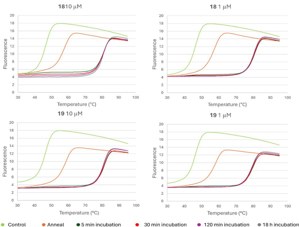
Fig. 5 Graphs showing DNA melting profiles after different incubation times of the DNA sequence (sequence 1) 5'-F-A<sub>7</sub>GA<sub>6</sub>T<sub>3</sub>-3'/5'-A<sub>5</sub>T<sub>6</sub>CT<sub>7</sub>-Q-3' with **18** and **19** at 10  $\mu$ M and 1  $\mu$ M, followed by annealing. Fluorescence is in arbitrary units.
