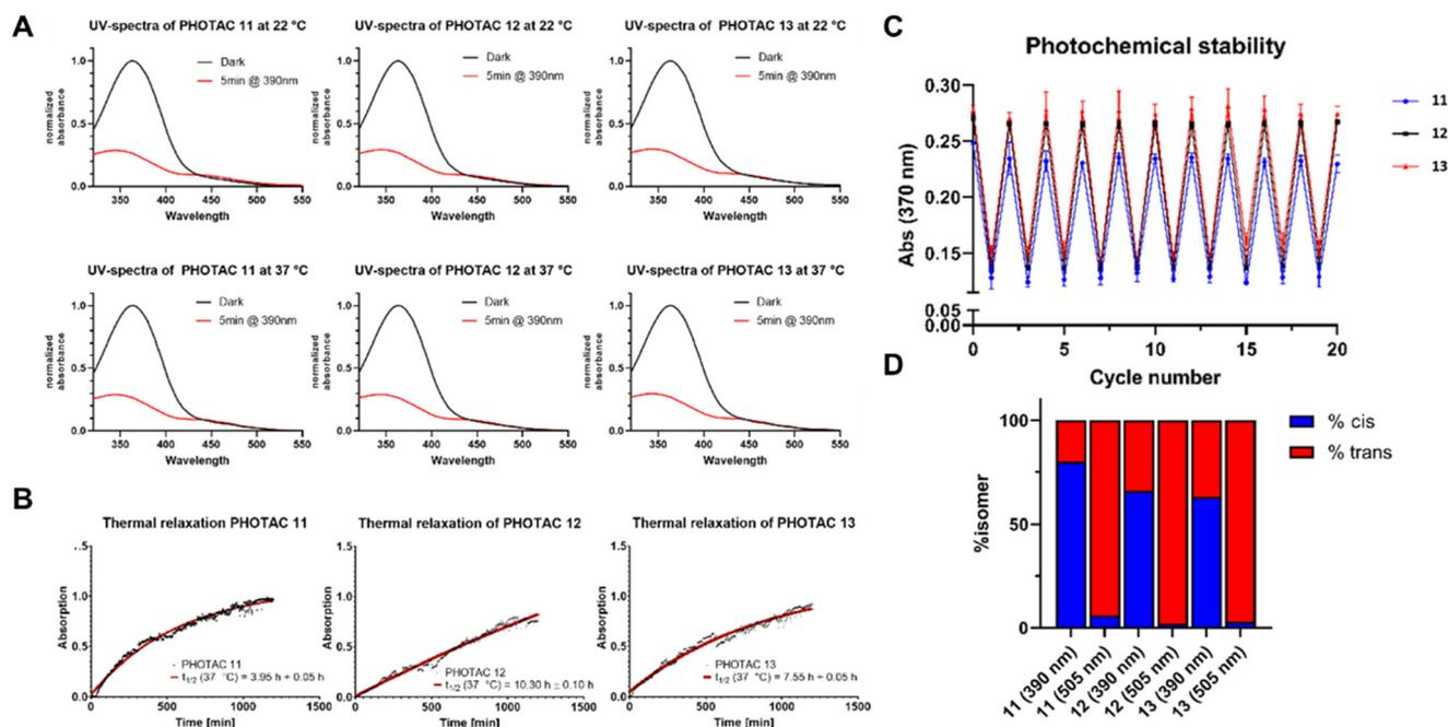
Fig. 3 (A) Overlaid UV-vis spectra of the *cis*- and *trans*-state PHOTACs **11–13** at 22 °C and 37 °C in DMSO. (B) Thermal relaxation measurements of the synthesized PHOTACs **11–13**. (C) Photochemical stability of the synthesized PHOTACs **11–13** over 20 cycles of switching between the *cis*- and the *trans*-isomer. (D) Percentage of *cis*- and *trans*-isomer of PHOTACs **11–13** after irradiation with 390 nm and 505 nm.
