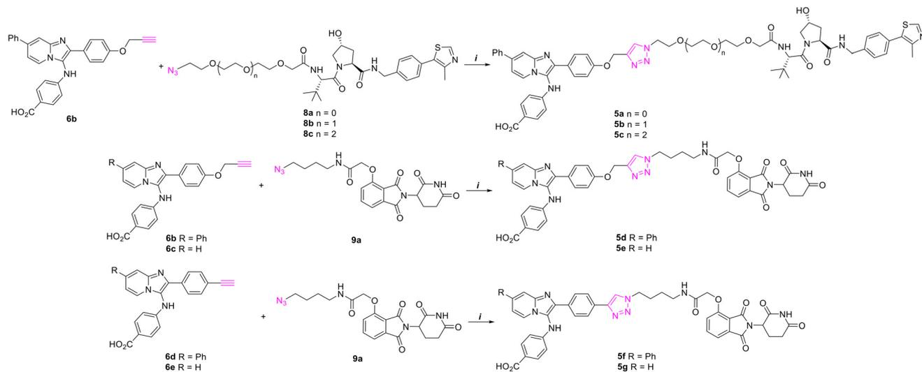
**Scheme 2** Synthesis of compounds **5a–5g** using CuAAC click reaction. Reagents and conditions: (i) TBTA,  $\text{CuSO}_4 \cdot 5\text{H}_2\text{O}$ , sodium L-ascorbate, DMSO,  $\text{H}_2\text{O}$ , rt.
