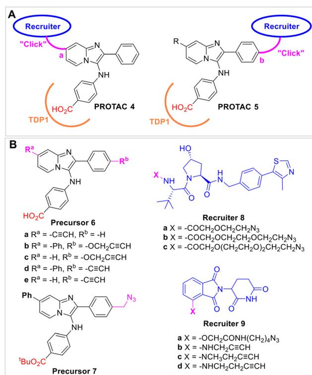
**Fig. 3** Design of TDP1 PROTACs that employ alkyne and azide precursors. (A) Structures of PROTACs (4 and 5) that append the recruiter linkers at the pyridine ring site "a" and the phenyl ring site "b" positions, respectively. (B) Structures of "click" functionality-bearing intermediates; phenyl imidazopyridine-derived TDP1-binding analogs (6a–6e and 7); and VHL-recruiter hydroxyproline-derived precursors (8a–8c) and CRBN-recruiter thalidomide-derived precursors (9a–9d).
