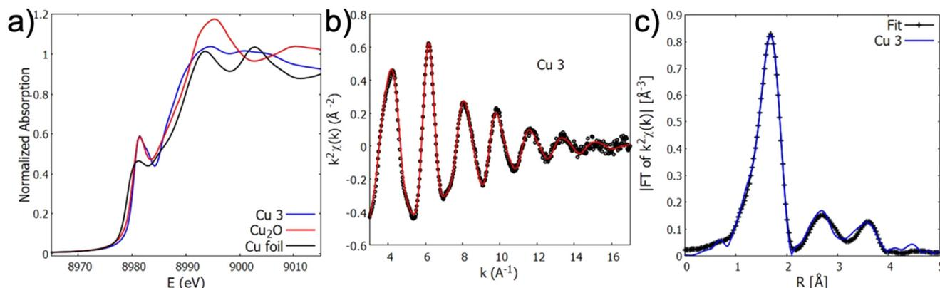
**Fig. 3** a) Normalized XANES spectrum of Cu K edge of **3** (blue), Cu<sub>2</sub>O (red) and Cu foil (black) as reference compounds. b)  $k^2$ -Weighted experimental (black) and fit (red) curves for **3**. c) Moduli of Fourier transforms (FT) of  $k^2\chi_{\text{exp}}(k)$  of experimental (blue) and best fit (black) curves; the FT curves have not been corrected for the phase shift effect, resulting in a main peak shift of approximately  $-0.5$  Å with respect to the actual distance.
