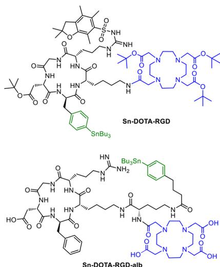
**Fig. 8** Molecule structures of the <sup>t</sup>Bu-protected RGD-stannyl precursor Sn-DOTA-RGD and the stannyl-precursor Sn-DOTA-RGD-alb with albumin binder.
