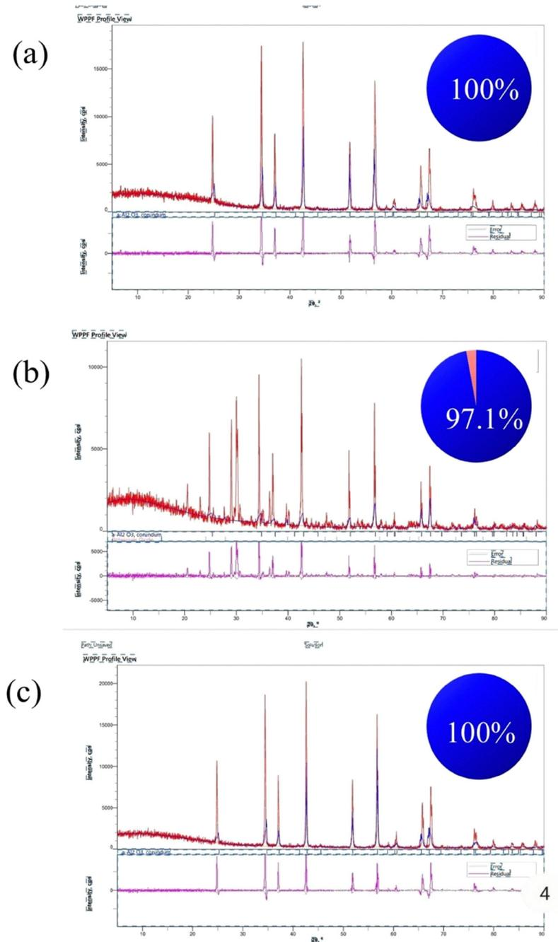
Fig. 2 Quantitative analysis of  $\alpha$ -alumina NPs by the WPPF method.
