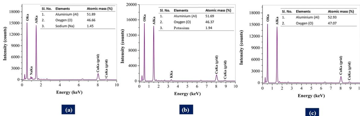
Fig. 11 EDS pattern of the synthesized  $\alpha$ -alumina NPs.
