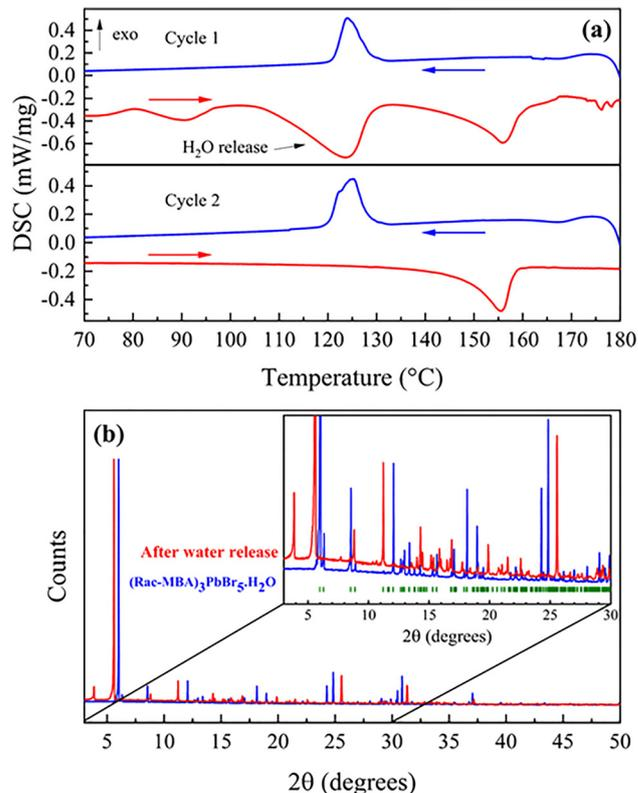
**Fig. 3** (a) DSC data of (Rac-MBA)<sub>3</sub>PbBr<sub>5</sub>·H<sub>2</sub>O performed at the first and second cycles. (b) Powder XRD of the as-grown (Rac-MBA)<sub>3</sub>PbBr<sub>5</sub>·H<sub>2</sub>O and the new phase after water release from thermal treatment, both at room temperature. Green tick marks in the inset represent the expected Bragg reflection positions considering a monoclinic phase with C2/c space group symmetry of the hydrated perovskite.
