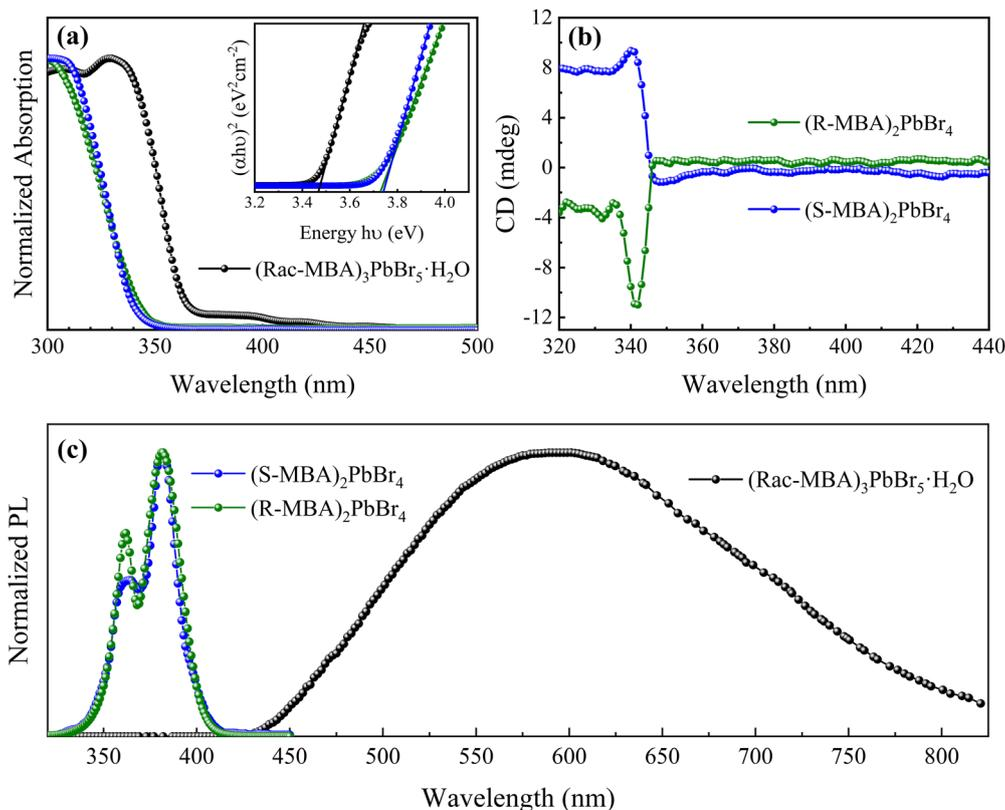
Fig. 5 Room-temperature optical properties of the (*R*-/*S*-MBA)<sub>2</sub>PbBr<sub>4</sub> and (Rac-MBA)<sub>3</sub>PbBr<sub>5</sub>·H<sub>2</sub>O perovskites. (a) Normalized absorption spectra with the Tauc plot in the inset. (b) Circular dichroism of the enantiomer-based perovskites. (c) Normalized photoluminescence spectra.
