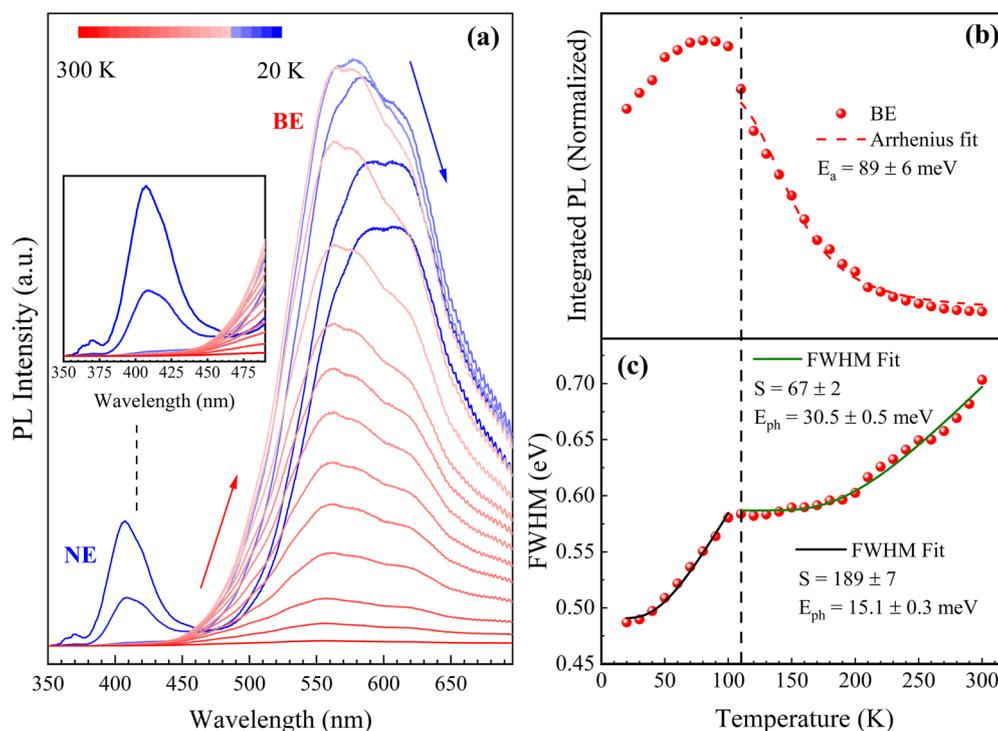
Fig. 6 (a) PL temperature dependence of (Rac-MBA)<sub>3</sub>PbBr<sub>5</sub>·H<sub>2</sub>O perovskites. (b) Normalized integrated PL intensity and (c) the FWHM of BE dependence on temperature.
