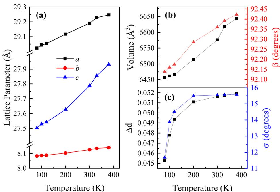
Fig. 7 Temperature dependence of the lattice parameters (a)  $a$ ,  $b$ ,  $c$ , and (b)  $\beta$  along with the unit cell volume of (Rac-MBA)<sub>3</sub>PbBr<sub>5</sub>·H<sub>2</sub>O perovskites. (c) Behavior of octahedral distortions evaluated using the distortion index  $\Delta d$  and bond angle variance  $\sigma$  with temperature.
