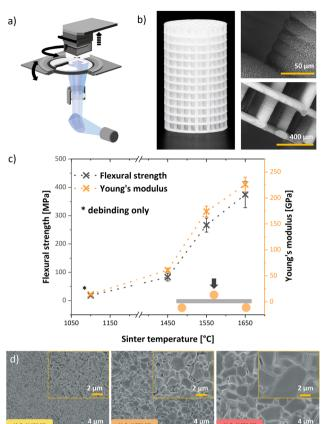
**Fig. 1** Printing set-up of lithography-based ceramic manufacturing (LCM) by Lithoz GmbH (a), sintered grid-like  $\alpha$ -alumina support structure ( $\emptyset$  = 2.5 mm, h = 5 mm) with MOF-functionalization (b), mechanical properties according to sinter temperature (c) and FE-SEM images of  $\alpha$ -alumina sintered at 1450 °C, 1550 °C and 1650 °C (d).
