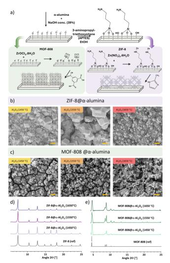
Fig. 2 Schematic functionalization of  $\alpha$ -alumina with MOF-808 and ZIF-8 (a). FE-SEM images of ZIF-8 (b) and MOF-808 (c) grown onto differently sintered  $\alpha$ -alumina. PXRD patterns of ZIF-8@ $\alpha$ -alumina (d) and MOF-808@ $\alpha$ -alumina (e).
