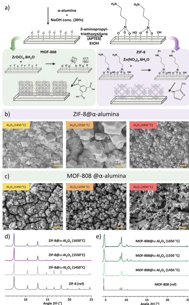
**Fig. 2** Schematic functionalization of  $\alpha$ -alumina with MOF-808 and ZIF-8 (a). FE-SEM images of ZIF-8 (b) and MOF-808 (c) grown onto differently sintered  $\alpha$ -alumina. PXRD patterns of ZIF-8@ $\alpha$ -alumina (d) and MOF-808@ $\alpha$ -alumina (e).
