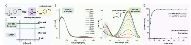
Fig. 3 DMNP degradation reaction (a),  $^{31}P$ -NMR Spectra of MOF-808@ $\alpha$ -alumina and  $\alpha$ -alumina before and after catalysis (b), UV-vis absorbance spectra of  $\alpha$ -alumina and MOF-808@ $\alpha$ -alumina during the reaction (c), and conversion based on p-nitrophenoxide formation (d)
