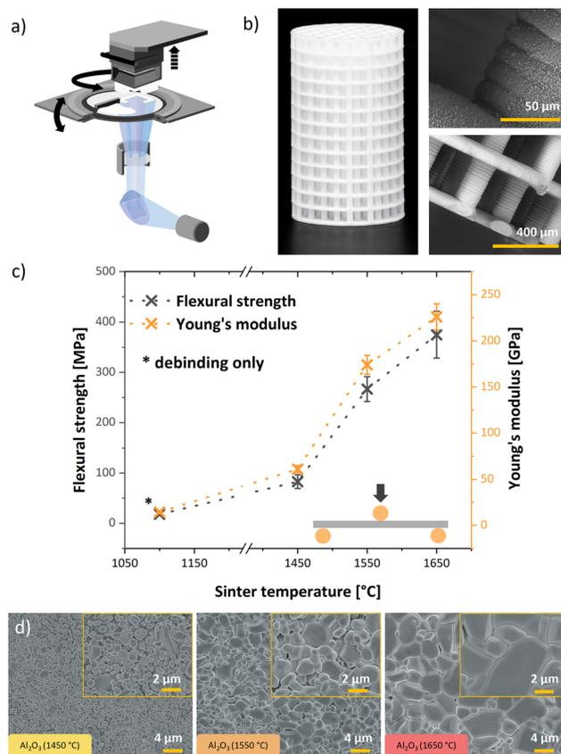
**Fig. 1** Printing set-up of lithography-based ceramic manufacturing (LCM) by Lithoz GmbH (a), sintered grid-like  $\alpha$ -alumina support structure ( $\varnothing = 2.5$  mm,  $h = 5$  mm) with MOF-functionalization (b), mechanical properties according to sinter temperature (c) and FE-SEM images of  $\alpha$ -alumina sintered at 1450 °C, 1550 °C and 1650 °C (d).
