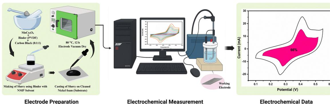
Fig. 2 Fabrication of AlV–MnCo<sub>2</sub>O<sub>4</sub> electrode and electrochemical testing process, including slurry preparation, coating on nickel foam, vacuum drying, and CV analysis in a three-electrode setup (created in Biorender.com).
