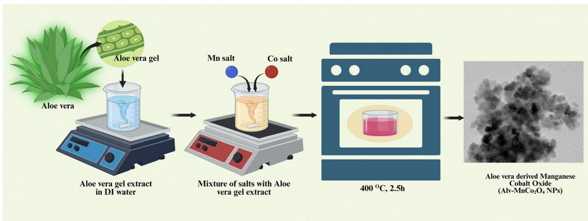
Fig. 1 Schematic representation of the green synthesis route for AlV–MnCo<sub>2</sub>O<sub>4</sub> NPs, involving Aloe vera extract preparation, precursor mixing, and thermal treatment to obtain the final nanomaterial (created in Biorender.com).
