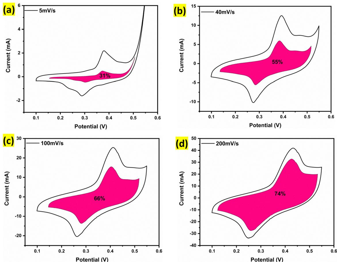
Fig. 8 Capacitive and diffusion contribution analysis of Al<sub>v</sub>-MnCo<sub>2</sub>O<sub>4</sub> N at different scan rates: (a) at  $5 \text{ mV s}^{-1}$ , capacitive contribution is 31% (b) at  $40 \text{ mV s}^{-1}$ , capacitive contribution is 55%; (c) at  $100 \text{ mV s}^{-1}$ , capacitive contribution is 66%; (d) at  $200 \text{ mV s}^{-1}$ , capacitive contribution increases to 74%, highlighting surface-dominated behavior at higher scan rates.
