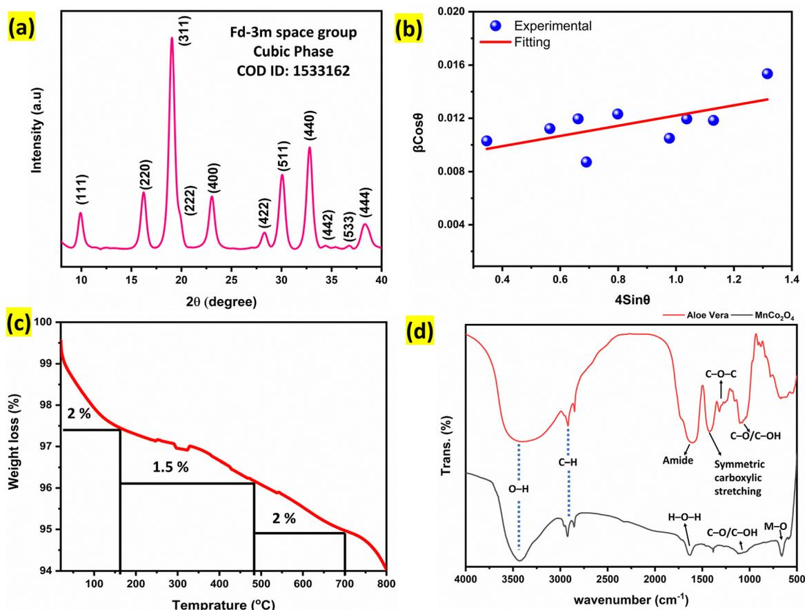
Fig. 3 (a) Synchrotron XRD pattern of AlV–MnCo<sub>2</sub>O<sub>4</sub> NPs recorded in transmission mode using a wavelength of 0.08262 nm. (b) Williamson–Hall plot used to calculate the crystallite size and microstrain in AlV–MnCo<sub>2</sub>O<sub>4</sub> NPs. (c) Thermogravimetric analysis (TGA) showing mass loss behaviour of the material. (d) FTIR spectra of Aloe vera extract (red line)<sup>34</sup> and AlV–MnCo<sub>2</sub>O<sub>4</sub> NPs (black line).
