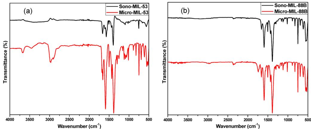
Fig. 2 FTIR spectra of (a) Fe-MIL-53 and (b) Fe-MIL-88B.
