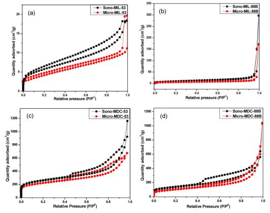
Fig. 6  $N_2$  adsorption-desorption isotherms of (a) Fe-MIL-53, (b) Fe-MIL-88B, (c) MDC-53 and (d) MDC-88B.
