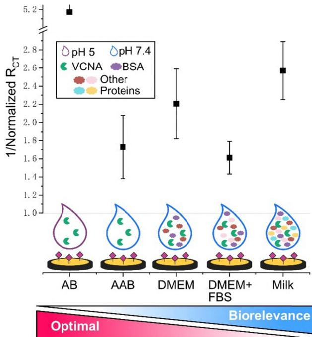
Fig. 3 Impedimetric response of the **AuE-H3** to VCNA conditions that vary from optimal (red) to biorelevant (blue). Response was measured in pH 5.0 (AB) or in pH 7.4 (AAB, DMEM, DMEM + FBS, milk). DMEM and DMEM + FBS represent two typical cell culture media that contain a large variety of proteins that might interfere with the biosensing. The normalized  $R_{CT}$  was calculated by dividing the response of the sialylated electrode by the response recorded after the exposure to VCNA.
