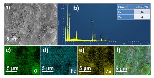
Fig. 4 SEM images (a), EDX spectra (b), corresponding EDX elemental maps (c)-(e), and an overlay of the EDX elemental map for ZDH4 (f).
