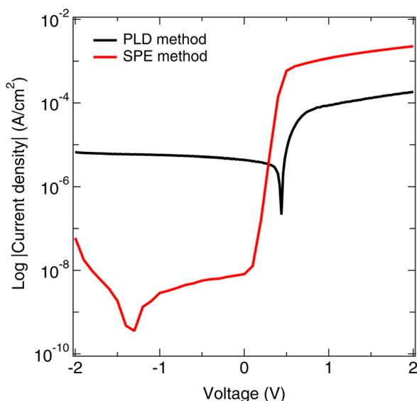
Fig. 6  $J$ - $V$  characteristics of Nb:BWO/ $\beta$ -Ga<sub>2</sub>O<sub>3</sub> pn junction diodes using Nb:BWO thin films prepared by PLD and SPE methods.
