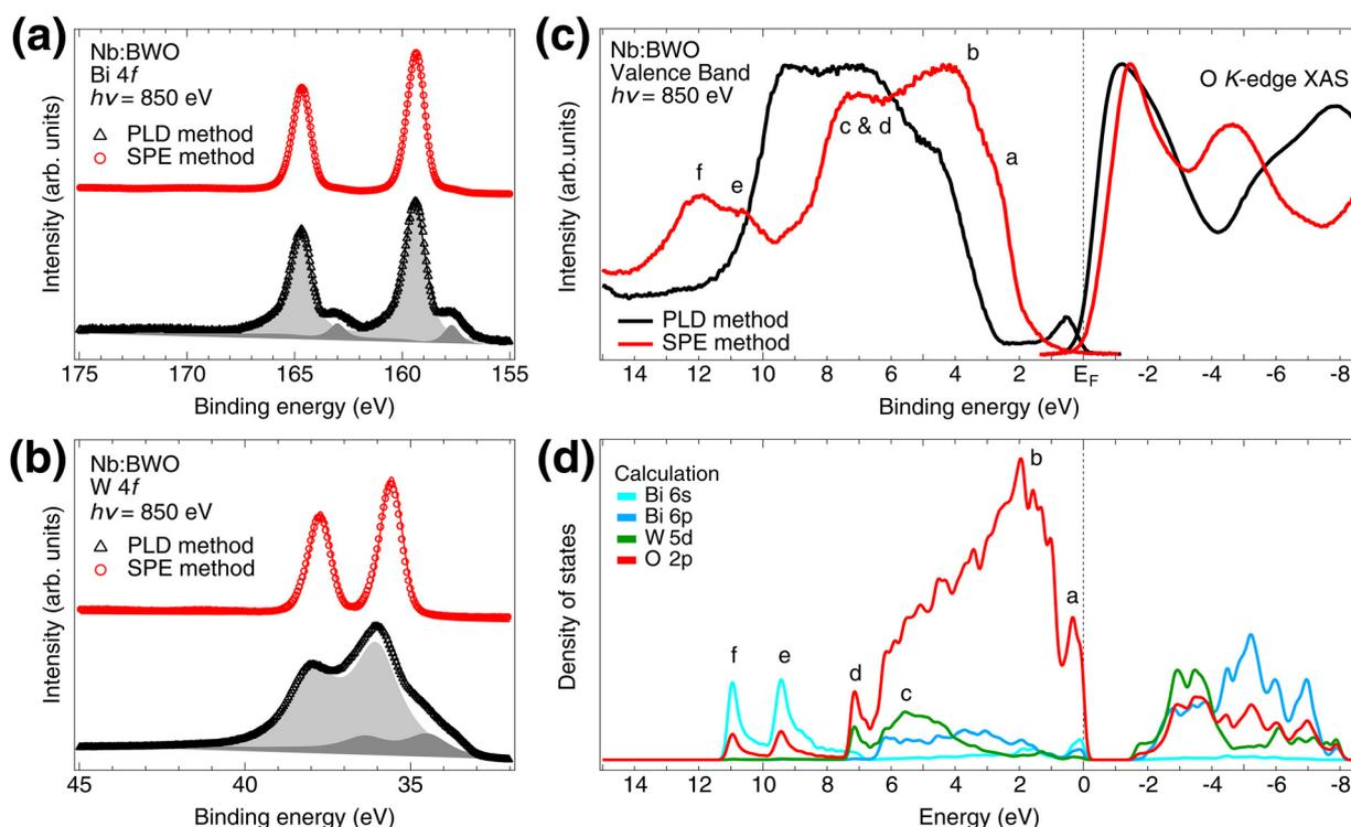
Fig. 5 (a) Bi 4f and (b) W 4f core-level spectra of PLD and SPE samples. (c) Valence band PES and O K-edge XAS spectra of PLD and SPE samples. (d) DOS of Bi<sub>2</sub>WO<sub>6</sub> from DFT simulations.
