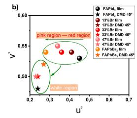
Fig. 5 (a) Chromaticity coordinates CIELAB ( $a^*$ ,  $b^*$ ), the rectangular region defines the coordinate range accepted for window Applications ( $-5 < a^* < 1$ and  $-5 < b^* < 5$ ), <sup>55</sup> (b) uniform chromaticity coordinate (CIELu'v'1976) for the net perovskite films and devices with DMD contact at 45° light incidence.
