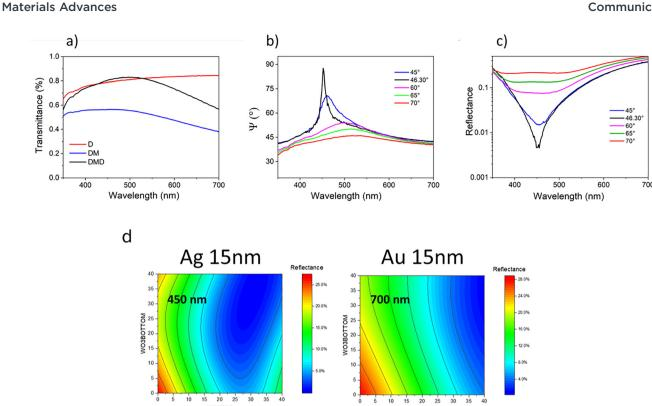
Fig. 1 (a) Transmittance spectra of produced D, DM, and DMD structures, acquired at normal incidence as a function of the incident wavelength. (b) Ellipsometric data of the  $\Psi$  phase of DMD40 at different angles of the incident light. (c)Total reflectance of DMD40 at different angles of the incident light. (d) The simulation maps of reflectance for different thicknesses of bottom and top dielectric layers using silver (Ag) and gold (Au), respectively.
