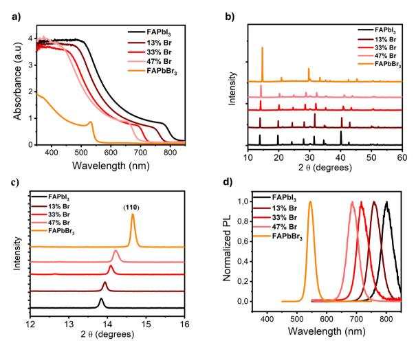
Fig. 2 (a) UV-Visible absorption spectra of mixed halide FAPbI<sub>3-x</sub>Br<sub>x</sub> perovskites thin films with different bromide concentration, (b) corresponding X-ray diffraction (XRD) patterns, (c) zoomed-in XRD pattern highlighting a shift in the peak position (110) with increasing Br content and (d) normalized photoluminescence spectra of mixed halide  $FAPbI_{3-x}Br_x$  perovskites thin films with different bromide concentration.
