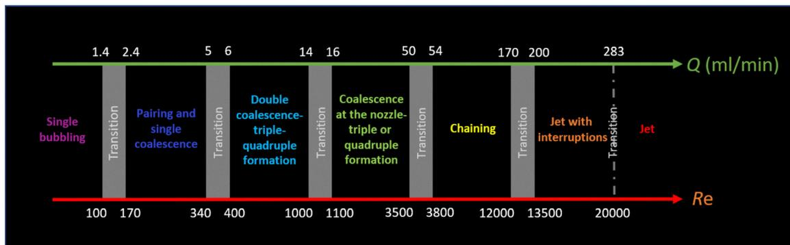
Fig. 7 Schematic for the transitions among different bubbling regimes from single bubbling ( $Re < 170$  and  $Q < 2.4 \text{ mL min}^{-1}$ ) to jetting ( $Re > 1200$  and  $Q > 170 \text{ mL min}^{-1}$ ). The names of the bubbling regimes were given by Kyriakides *et al.* in ref. 45.
