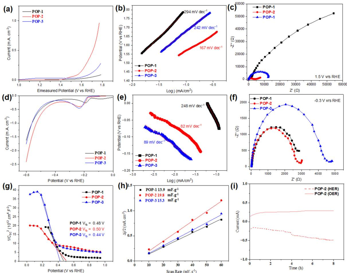
Fig. 4 (a) and (d) LSV curves, (b) and (e) Tafel slopes, and (c) and (f) EIS measurements for the OER and HER, respectively, and (g) Mott–Schottky plot for POP-1, POP-2 and POP-3. (h) The  $C_{dl}$  values to evaluate the ECSA and (i) CA stability over 8 hours of POP-2.
