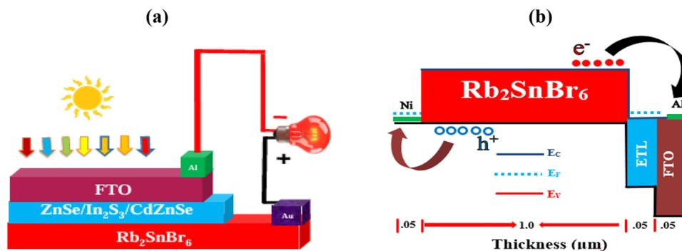
Fig. 1 Al/FTO/ETL/Rb<sub>2</sub>SnBr<sub>6</sub>/Au diagram illustration (a) and band sketch (b).
