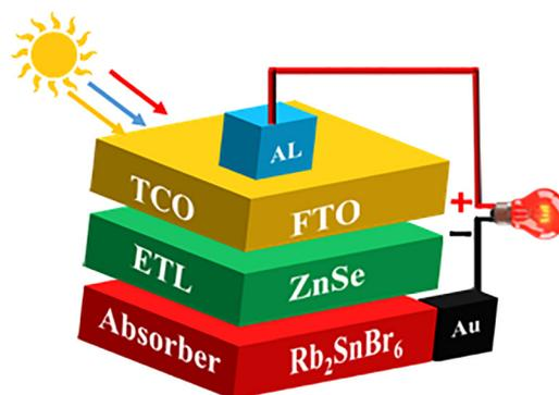
Fig. 14 The optimum structure Al/FTO/ZnSe/ $\text{Rb}_2\text{SnBr}_6$ /Au.
