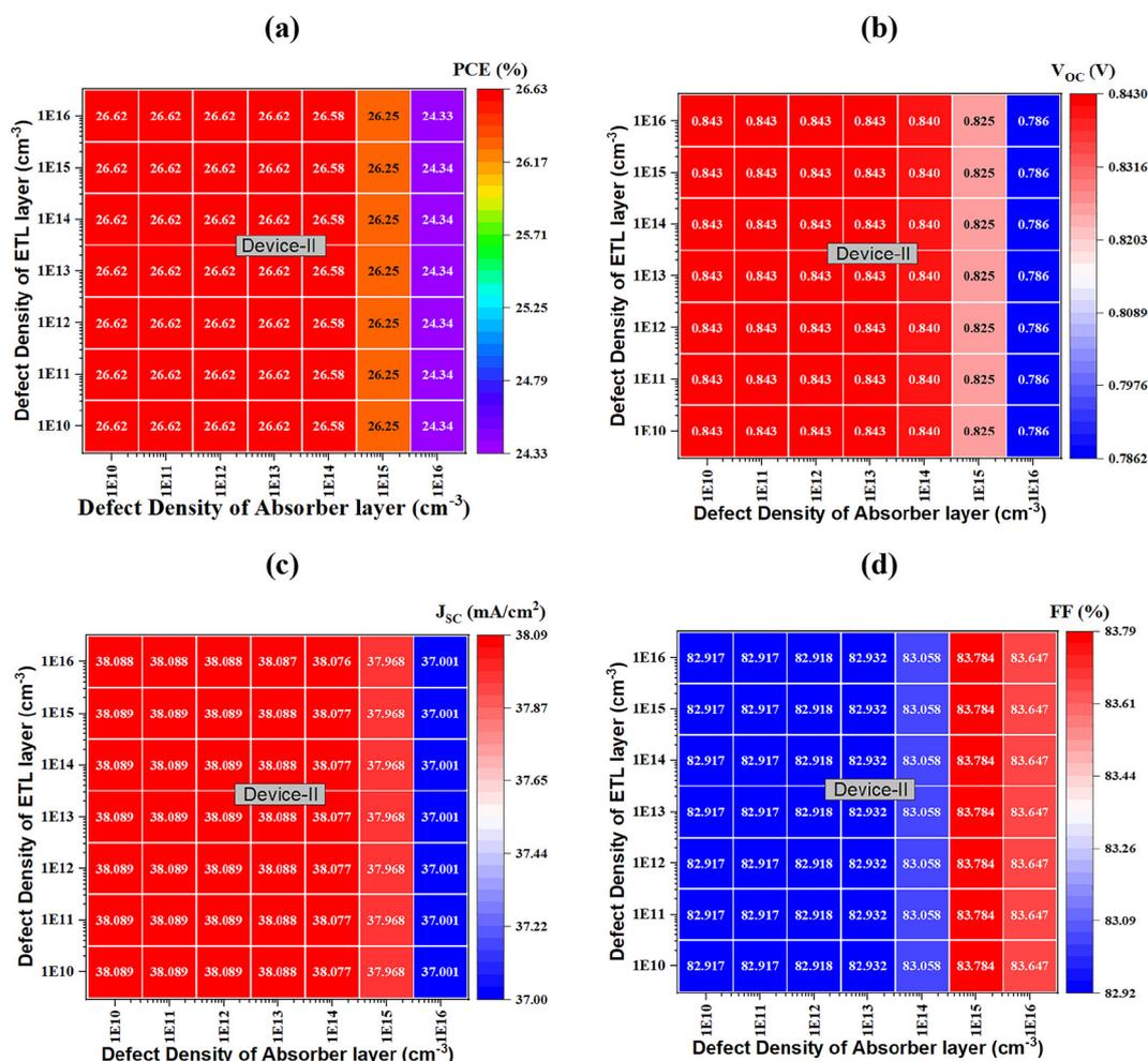
Fig. 8 Role of PV factors considering the modification in the defect density of the ETL vs. absorber layer for device-II: (a) efficiency, (b)  $V_{\text{OC}}$ , (c)  $J_{\text{SC}}$ , and (d) FF.
