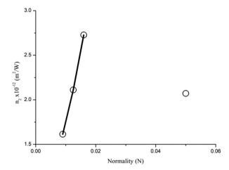
Fig. 12 Normality dependence of  $n_2$  for KMnO<sub>4</sub>
