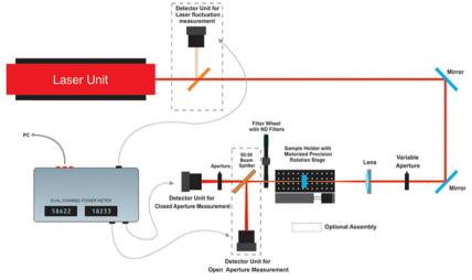
Fig. 2 Z-scan experimental setup
