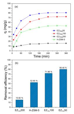
Fig. 2 Time-dependent adsorption of MB onto different adsorbents (a) and (b) removal efficiency for each material after 4 h of contact time. Experimental conditions: initial MB concentration =  $50 \text{ mg L}^{-1}$ , adsorbent dosage = 25 mg, V = 50 mL, pH (unadjusted) = 5.6, 0.01 M NaCl, stirring speed = 250 rpm and T = 25 °C.
