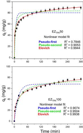
Fig. 8 Non-linear pseudo-first, pseudo-second, and Elovich model fit for  $EZ_{TPA}50$  and  $EZ_{TPA}100$ . Experimental conditions: adsorbent dosage 25 mg, solution volume 50 mL, background electrolyte = 0.01 M NaCl, pH = 7, T = 25 °C, stirring speed 250 rpm.
