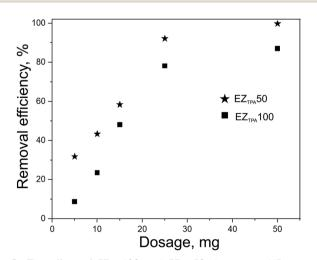
Fig. 5 The effect of  $EZ_{TPA}100$  and  $EZ_{TPA}50$  dosage on MB removal efficiency. Experimental conditions: initial MB concentration = 50 mg  $L^{-1}$ , V = 50 mL, pH = 7, 0.01 M NaCl, stirring speed = 250 rpm, T = 25 °C and time = 4 h.
