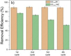
Fig. 10 Adsorbents' appearance before and after the first regeneration cycle performed at 550 °C for 4 h (a) and (b) removal efficiencies of EZ<sub>TPA</sub>50 and EZ<sub>TPA</sub>100 after four regeneration cycles at optimal conditions.
