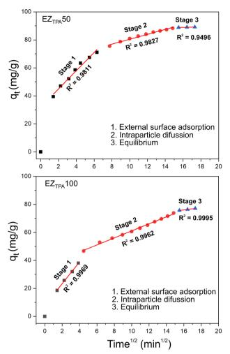
Fig. 9 Intraparticle diffusion model fit (Weber-Morris model) for EZ<sub>TPA</sub>100 and EZ<sub>TPA</sub>50.
