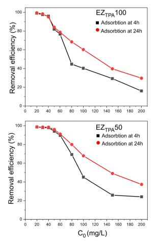
Fig. 6 Removal efficiency of methylene blue as a function of initial concentration ( $C_0$ ) after adsorption on EZ<sub>TPA</sub>100 (left) and EZ<sub>TPA</sub>50 (right) at contact times of 4 h (black squares) and 24 h (red circles). Experimental conditions: adsorbent dosage 25 mg, solution volume 50 mL, background electrolyte = 0.01 M NaCl, pH = 7, T = 25 °C, stirring speed 250 rpm.
