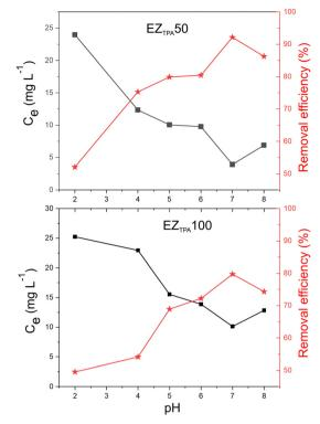
Fig. 4 Effect of different values of initial pH on the adsorption of MB onto EZTPA50. Experimental conditions: initial MB concentration =  $50 \text{ mg L}^{-1}$ , adsorbent dosage = 25 mg, V = 50 mL, 0.01 M NaCl, stirring speed = 250 rpm, T = 25 °C and time = 4 h.
