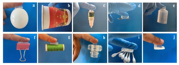
Fig. 6 The photos of polyacrylamide-LiCl ionic plain hydrogel adhere to different substrates. (a) Rubber ball; (b) paper cup; (c) plastic bottle; (d) aluminum scissors; (e) plastic cup; (f) Sn (tin) clip; (g) yarn bobbin; (h) glass made bottle cap; (i) wood made cotton butt; and (j) woven fabric.
