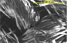
Fig. 2 (a) The microstructure of the PAAM-LiCl hydrogel; (b) untreated woven fabric.
