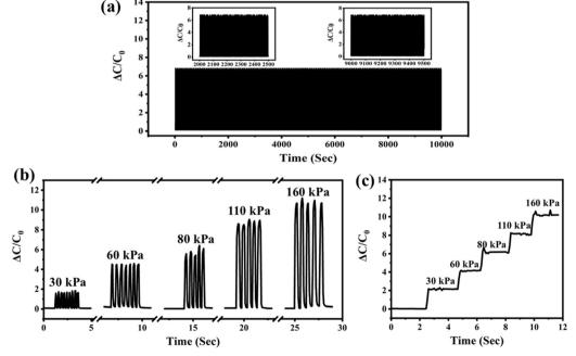
Fig. 4 Performance of woven fabric-based ionic plain hydrogel pressure sensor: (a) cycle for woven electrode; (b) gradient pressure for dynamic; (c) gradient pressure for static
