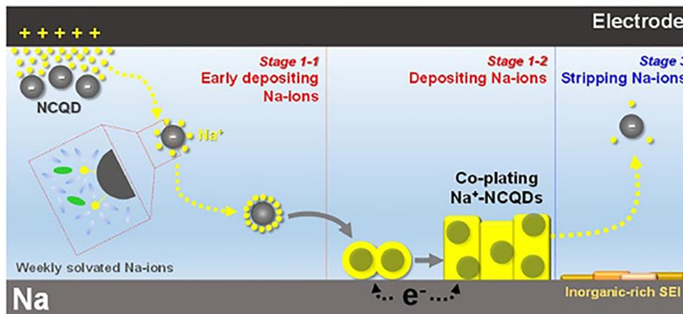
Fig. 25 Mechanism of N-CDs in regulating  $\text{Na}^+$  deposition/stripping behavior and stabilizing the SEI in SIBs.<sup>205</sup> Copyright 2025, Elsevier.
