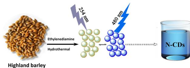
Fig. 4 Hydrothermal synthesis of N-CDs from highland barley.<sup>39</sup> Copyright 2019, MDPI.
