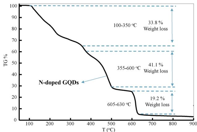
Fig. 20 TGA curve showing the thermal decomposition profile of N-doped GQDs.<sup>117</sup> Copyright 2019, Elsevier.
