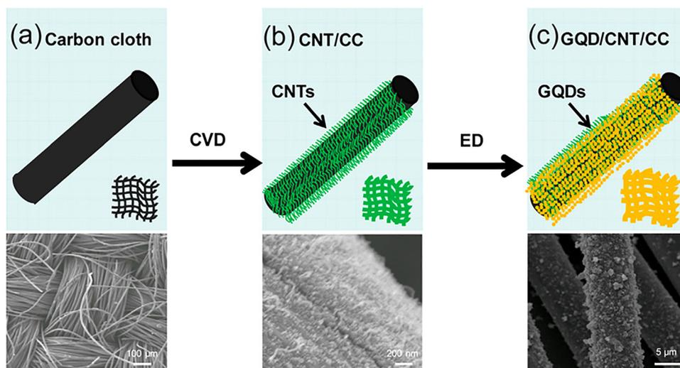
**Fig. 33** Schematic illustration for the preparation of 3D N-O-GQD/CNT/CC electrodes. (a) Pristine carbon cloth (CC) substrate. (b) CNTs grown on CC via CVD to form CNT/CC composite. (c) N-O-GQDs electrodeposited on CNT/CC to yield the final 3D N-O-GQD/CNT/CC electrode. Bottom panels show corresponding SEM images at different magnifications.<sup>265</sup> Copyright 2017, Elsevier.
