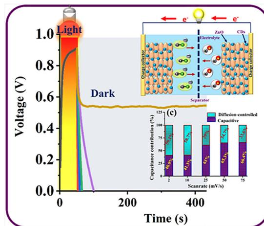
Fig. 30 Electrochemical performance characterization of the ZnO/N-CD composite supercapacitor electrode.<sup>253</sup> Copyright 2023, American Chemical Society.
