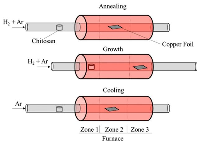
Fig. 8 Schematic illustration of the CVD synthesis process for N-GQDs.<sup>52</sup> Copyright 2018, American Chemical Society (ACS).
