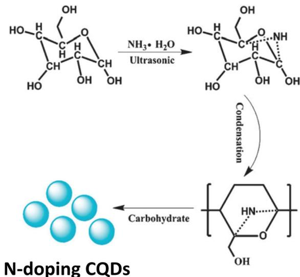
Fig. 11 Schematic representation of the ultrasonic synthesis process for N-CQDs from glucose precursors.<sup>78</sup> Copyright 2012, Royal Society of Chemistry.
