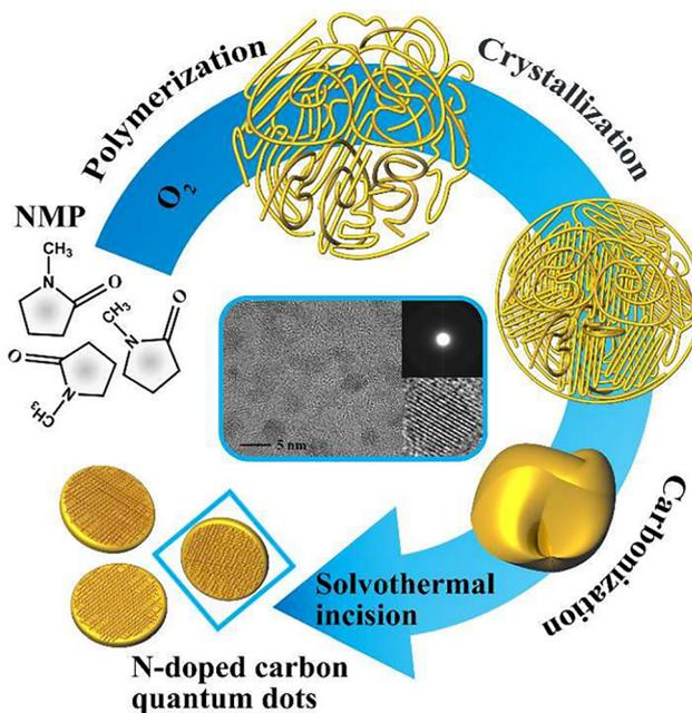
Fig. 5 One-step solvothermal synthesis of N-CDs from *N*-methylpyrrolidone (NMP).<sup>40</sup> Copyright 2016, Royal Society of Chemistry.
