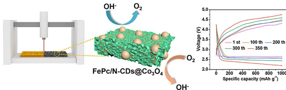
Fig. 27 Schematic illustration and electrochemical performance of FePc/N-CDs@Co<sub>3</sub>O<sub>4</sub> cathode for lithium–oxygen batteries.<sup>218</sup> Copyright 2022, Springer.
