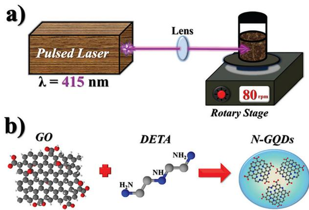
Fig. 9 Schematic illustration of (a) the pulsed laser ablation setup for N-GQD synthesis and (b) the DETA-mediated N-GQD formation process.<sup>64</sup> Copyright 2017, Royal Society of Chemistry.
