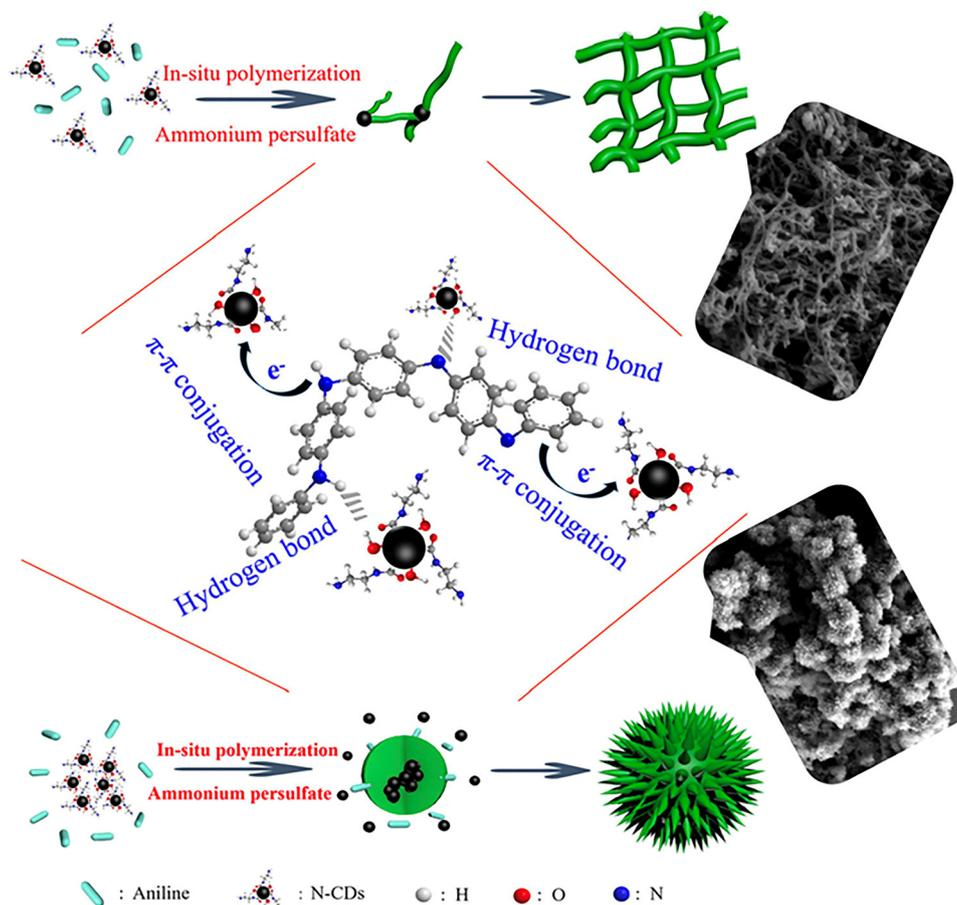
Fig. 29 Schematic illustration of the *in situ* oxidative polymerization process for N-CDs@PANI hybrid fabrication.<sup>243</sup> Copyright 2014, Wiley.
