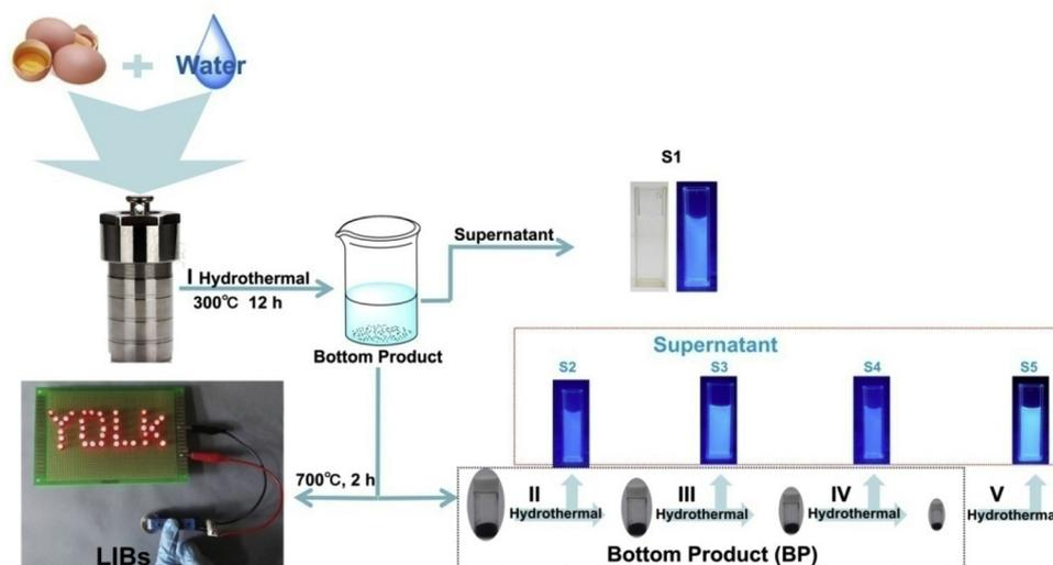
Fig. 24 Schematic illustration of the green hydrothermal synthesis process for N-CDs and derived bulk carbon anode materials for LIB applications.<sup>195</sup> Copyright 2018, Elsevier.
