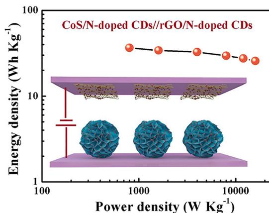
Fig. 31 Schematic illustration of the CoS/N-CDs/rGO hybrid supercapacitor electrode showing synergistic enhancement mechanisms.<sup>255</sup> Copyright 2020, Elsevier.
