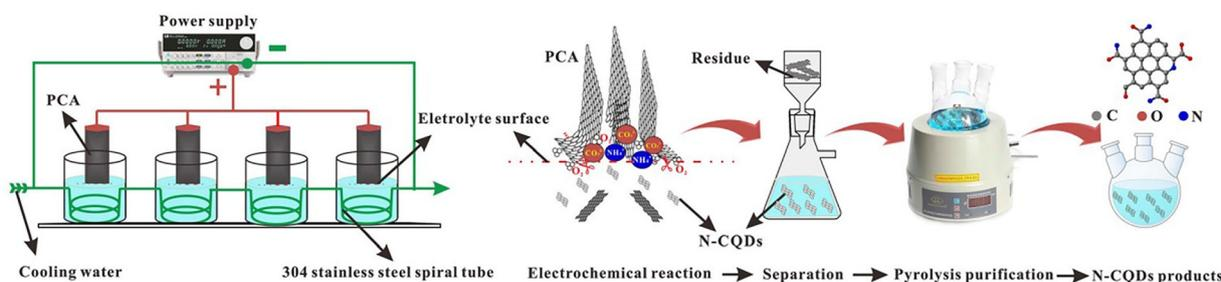
Fig. 10 Schematic depiction of the electrochemical exfoliation apparatus for the N-CQDs-related experimental device.<sup>73</sup> Copyright 2021, Springer.
