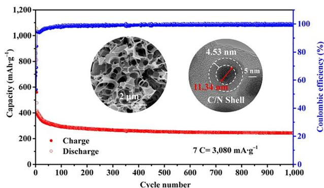
Fig. 26 Long-term cycling stability and structural integrity of the N-CQD-enhanced FeSb composite anode in PIBs.<sup>206</sup> Copyright 2022, Springer.
