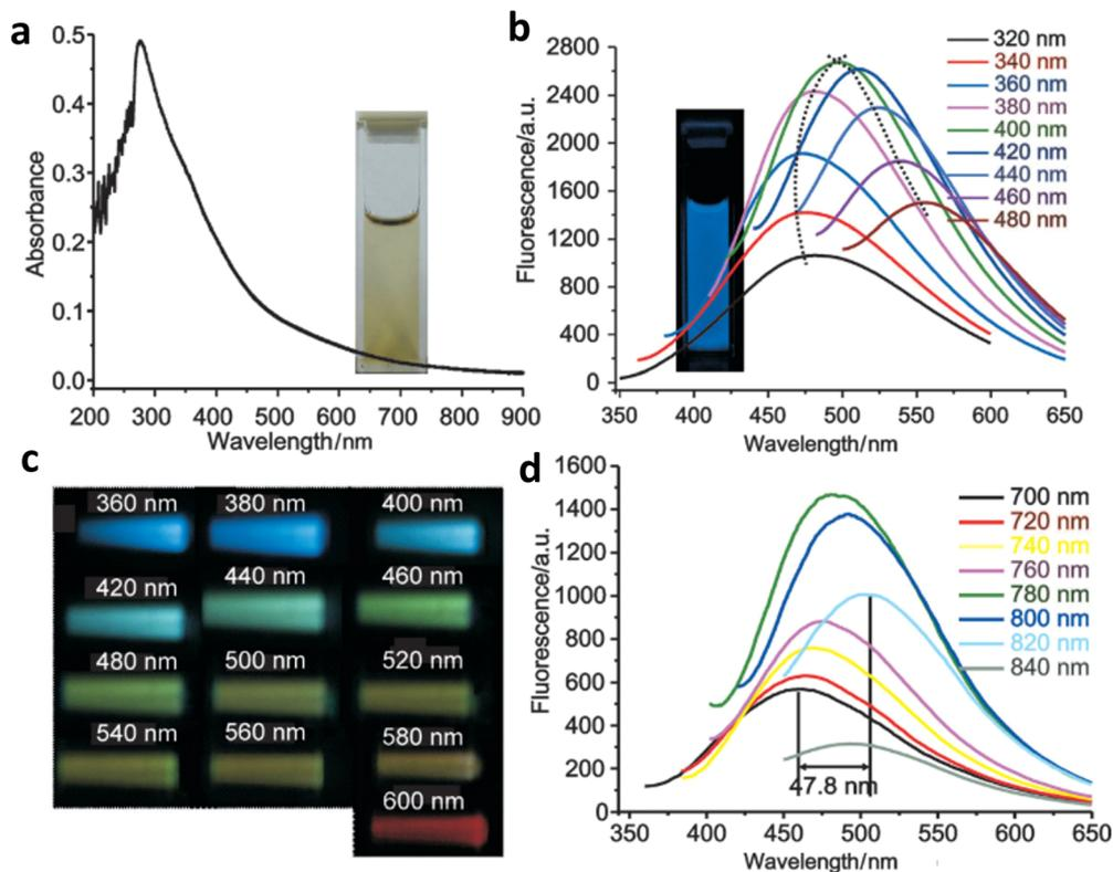
**Fig. 18** (a) UV-Vis absorption spectra of N-CDs with an inset showing solution appearance. (b) Excitation-dependent photoluminescence spectra featuring inset emission under 380 nm excitation. (c) Fluorescence microscopy images captured at different excitation wavelengths. (d) Up conversion photoluminescence spectra demonstrating anti-Stokes emission properties.<sup>109</sup> Copyright 2013, Wiley.
