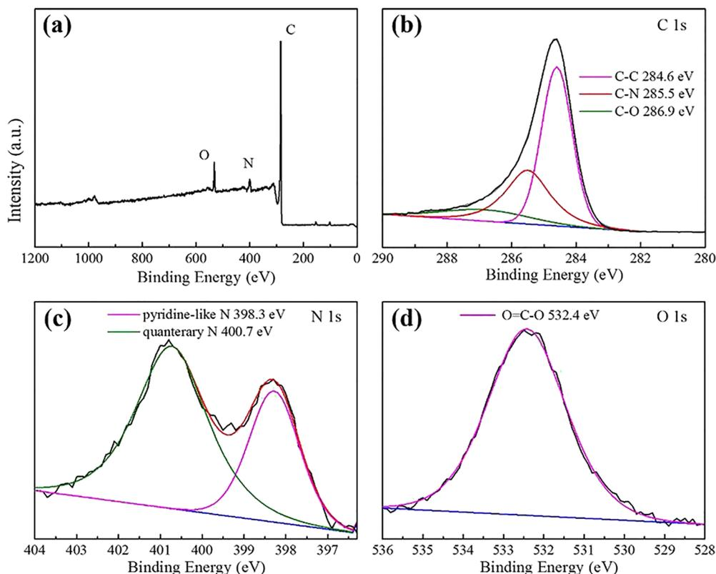
Fig. 17 XPS analysis of N-CDs annealed at 800 °C: (a) survey scan confirming C/N/O presence, (b) detailed C 1s spectrum, (c) high-resolution N 1s signal, and (d) O 1s peak analysis.<sup>40</sup> Copyright 2016, Royal Society of Chemistry.
