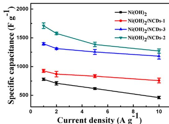
Fig. 28 Electrochemical performance of Ni(OH)<sub>2</sub>/N-CDs composite electrodes in hybrid supercapacitor applications.<sup>225</sup> Copyright 2019, Elsevier.
