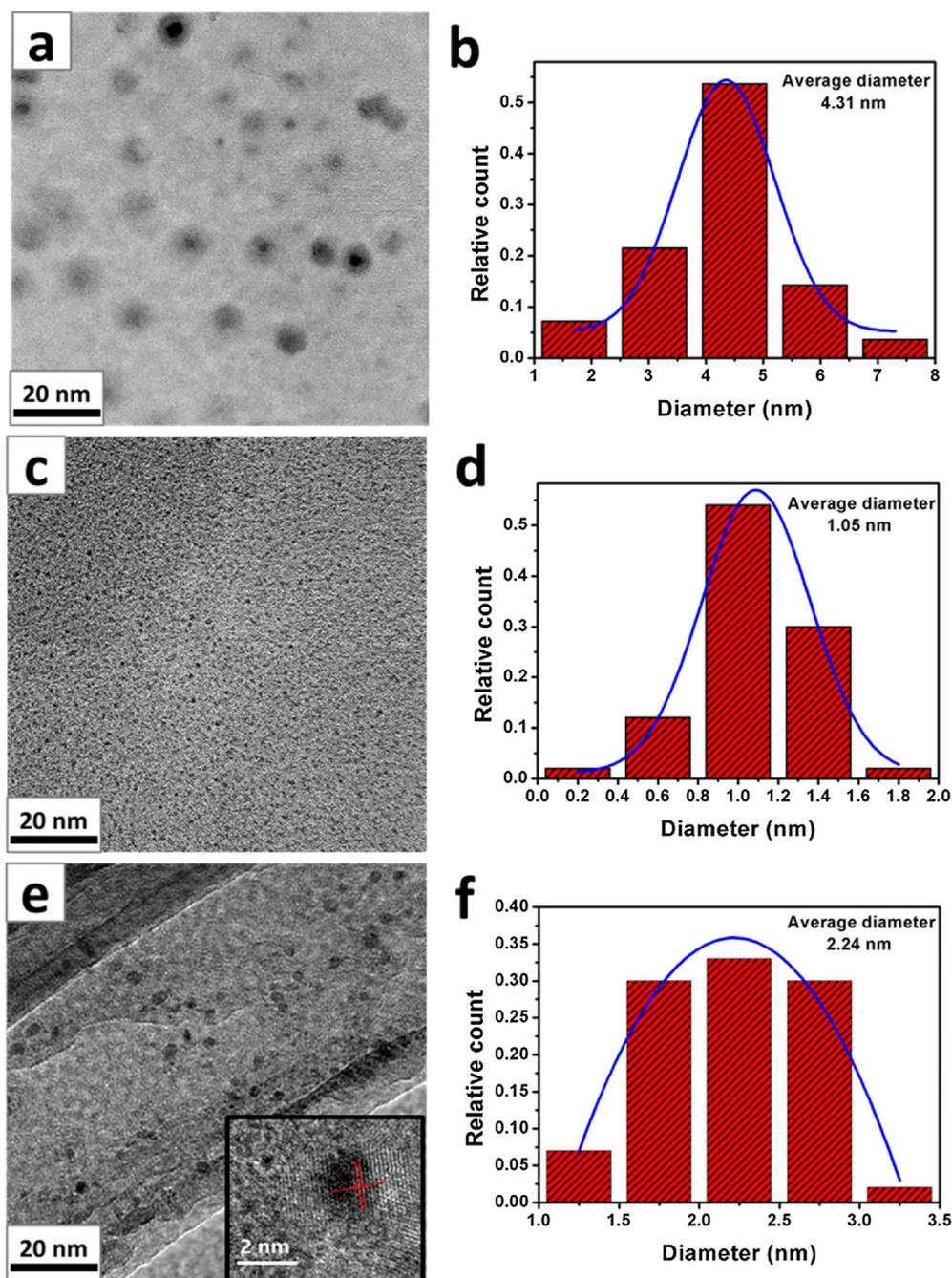
Fig. 19 TEM images and corresponding particle size distributions of (a) and (b) N-CDs160-1, (c) and (d) N-CDs200-1, and (e) and (f) N-CDs200-2.<sup>44</sup> Copyright 2017, Elsevier.
