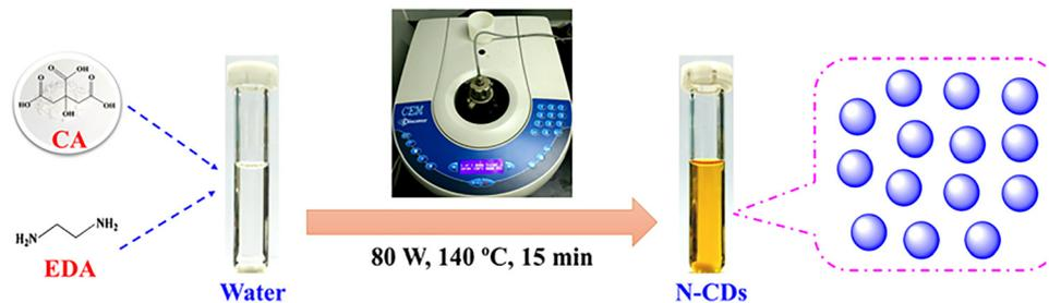
Fig. 7 Single-step microwave synthesis of photoluminescent N-CDs.<sup>48</sup> Copyright 2017, Springer.
