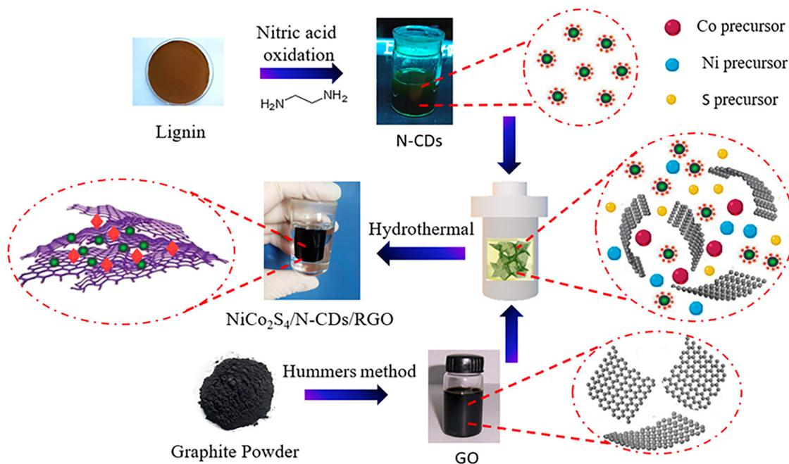
Fig. 32 Fabrication schematic of the  $\text{NiCo}_2\text{S}_4/\text{N-CDs}/\text{RGO}$  ternary hydrogel composite.<sup>256</sup> Copyright 2017, MDPI.
