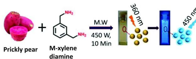
Fig. 6 Microwave-assisted synthesis of N-CDs from prickly pear and *m*-xylenediamine.<sup>47</sup> Copyright 2021, Royal Society of Chemistry.
