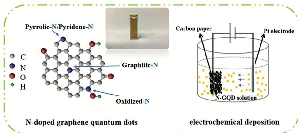
Fig. 23 Schematic illustration of N-GQDs and their electrochemical deposition process for supercapacitor applications.<sup>174</sup> Copyright 2018, Royal Society of Chemistry.
