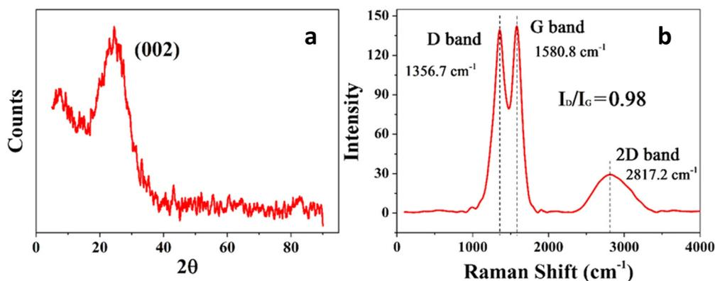
Fig. 15 (a) XRD pattern and (b) Raman spectrum of N-CDs.<sup>106</sup> Copyright 2025, Springer.
