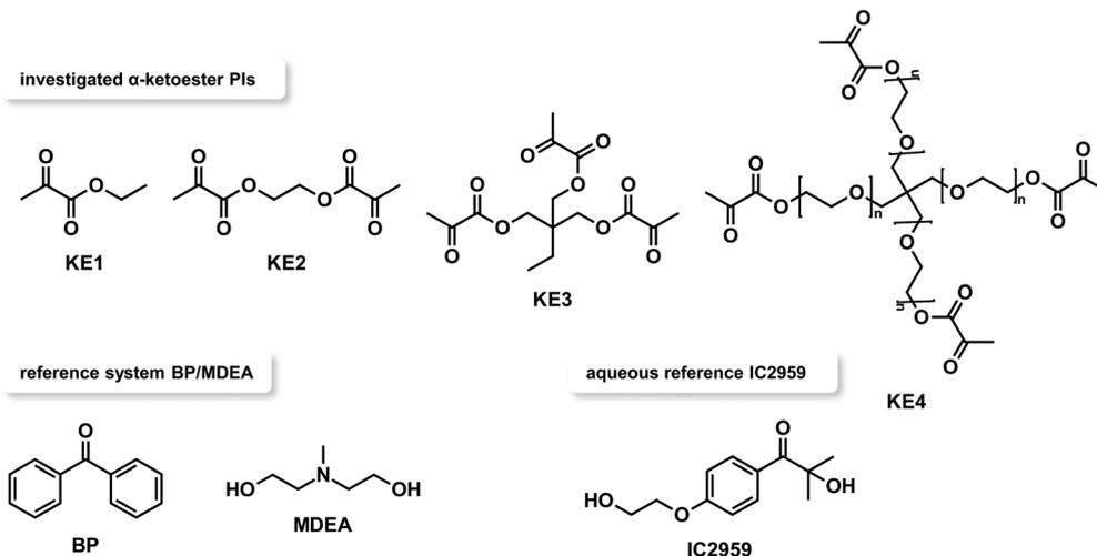
Fig. 3 Schematic representation of the photoinitiators: ethyl pyruvate (KE1), ethylene glycol dipyrivate (KE2), trimethylol propane tripyruvate (KE3), and ethoxylated pentaerythritol tetrapyrivate (KE4). The reference system for bulk (meth)acrylates consists of benzophenone (BP) and methyldiethanolamine (MDEA), whereas Irgacure 2959 (IC2959) was used as a reference in aqueous systems.
