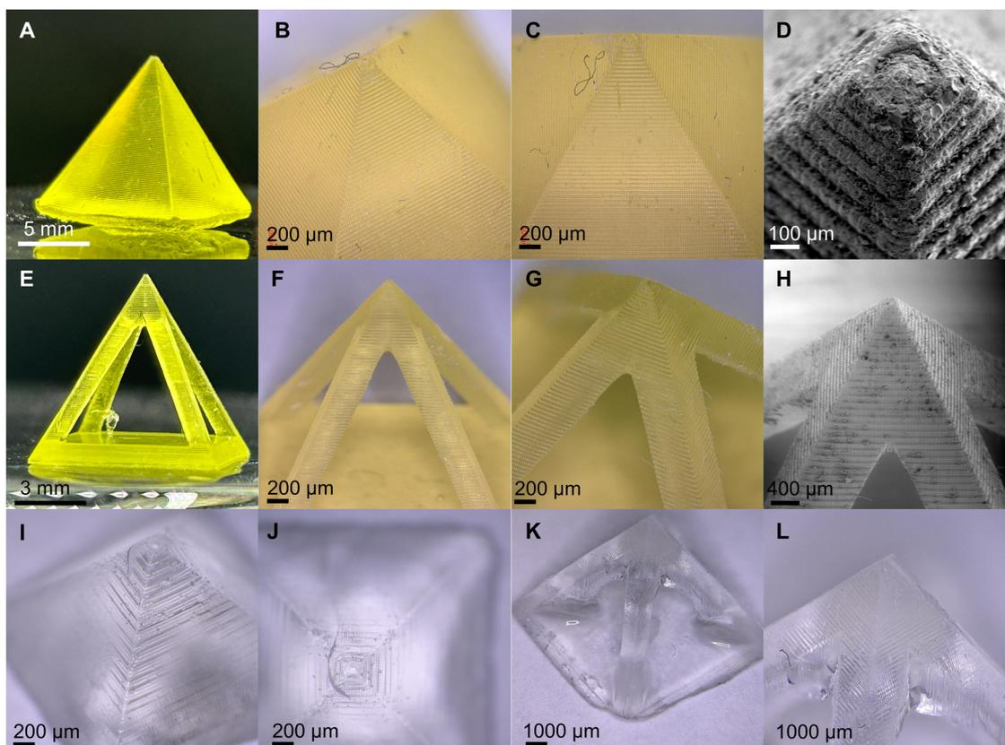
**Fig. 11** Light-(LM) and scanning electron microscopic (SEM) images of structures printed of 2 FG% KE3 in various monomers. (A)–(C) LM and (D) SEM of square pyramids (2 FG% KE3 in ethoxylated TMPTA + 0.02 wt% QY), (E)–(G) LM and (H) SEM of hollow square pyramids (2 FG% KE3 in ethoxylated TMPTA + 0.02 wt% QY). LM images of 3D structures of hydrogels (2 FG% KE3 in 50 wt% aqueous PEGDA): (I) and (J) square pyramid and (K) and (L) hollow square pyramid.
