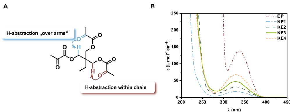
Fig. 4 (A) Proposed H-abstraction within the multifunctional  $\alpha$ -ketoester KE3: “traditional” H-abstraction within the same chain (red) and over the arms of the core molecule (blue). (B) UV-Vis spectra of the reference BP and ketoesters KE1–KE4 in acetonitrile ( $1 \times 10^{-2}$  M).
