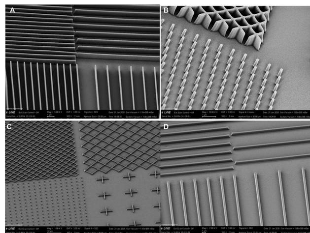
Fig. 10 SEM images of imprinted structures *via* UV-NIL. (A) and (B): resin JR NILcure (aliphatic diacrylate) containing 1 wt% KE3 as PI and (C), (D): hydrogel (50 wt% M286 in water) containing 1 wt% KE3 as PI.
