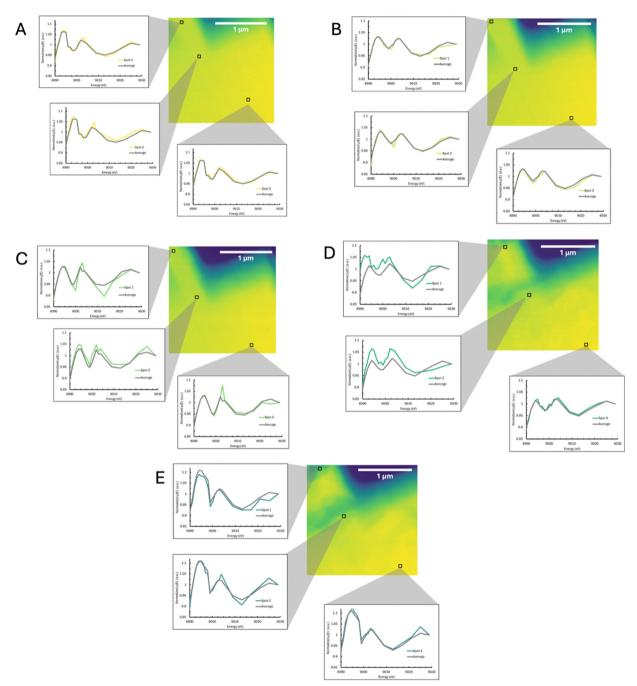
Fig. 2 Post-edge nano-XANES spectra at varying spots at (A) 31 °C, (B) 155 °C, (C) 280 °C, (D) 400 °C, and (E) 31 °C after heating. The average spectrum for each full sample at the respective temperature is shown with a grey line, the colored line represents the spectrum at the indicated point. Significant spectral differences are shown at each temperature. The scale bar in each XANES image represents  $\sim 1 \mu m$ .
