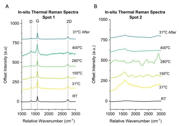
Fig. 4 In situ thermal Raman spectra at varying temperature points for spot 1 (A) and for spot 2 (B). The grey vertical lines (left) represent the D (1350 cm<sup>-1</sup>), G (1580 cm<sup>-1</sup>), and 2D (2700 cm<sup>-1</sup>) peaks of sp<sup>2</sup> hybridized carbon. Raman peaks are consistent for spot 1 whereas no clear Raman peaks are present at spot 2 for any temperature.
