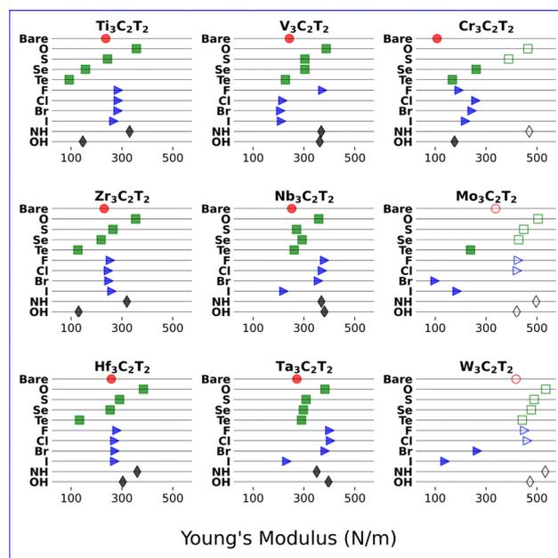
Fig. 9 Young's modulus ( $\text{N m}^{-1}$ ) for MXenes in their most stable configurations. Red circles are bare structures, green squares have terminations from chalcogens, blue triangles have terminations from halogens, while black diamonds are  $-OH$  and  $-NH$  terminations. Hollow markers indicate an ABA configuration, while solid markers indicate an ABC configuration.
