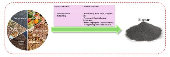
Fig. 6 Strategy for converting biomass into biochar.
