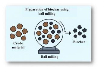
Fig. 5 Ball milling synthesis of biochar.
