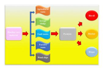
Fig. 4 Schematic diagram of biochar fabrication from multiple biomass sources through pyrolysis.
