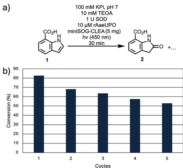
Fig. 4 (a) Reaction scheme and conditions for the blue-light mediated oxidation of **1** (1 mM) to oxindole **2** using rAaeUPO and *in situ* produced H<sub>2</sub>O<sub>2</sub> from miniSOG-CLEA. (b) Recyclability test of the miniSOG-CLEA photocatalyst.
