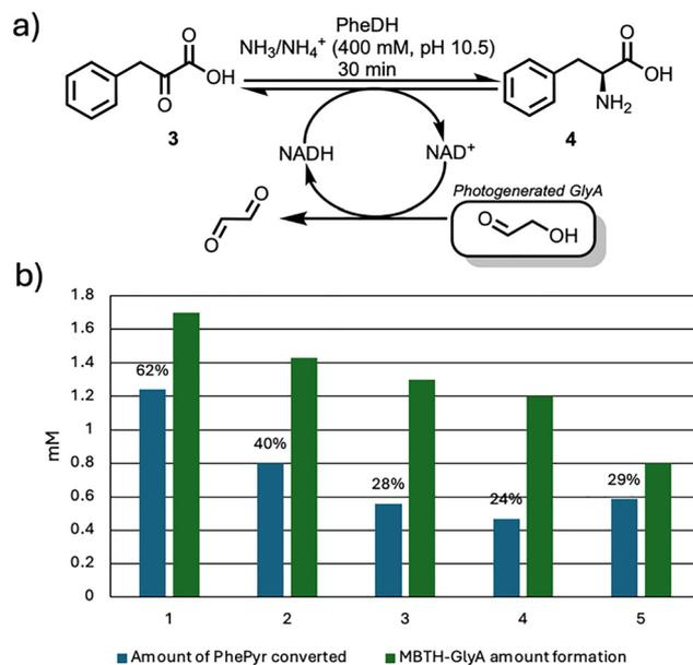
Fig. 6 Coupling photogenerated glycolaldehyde to PheDH-catalysed reductive amination. (a) Reaction scheme. (b) Recycling study (five 30-min irradiation cycles; 5 mg CLEA, 0.5 M TEOA, 0.2 mM NAD<sup>+</sup>, in 1 mL). Blue bars: PhePy converted (%) green bars: GlyA formed (mM, quantified as MBTH adduct). Product formation parallels GlyA availability. No product was detected in “no-light” or “no-CLEA” controls.
