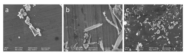
Fig. 4 SEM micrographs of (a) ZnS nanoparticles, (b) CoS nanoparticles, and (c) optimized mixed ZnS-CoS nanoparticles, illustrating the surface morphology of the synthesized materials.
