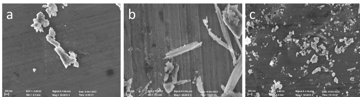
Fig. 4 SEM micrographs of (a) ZnS nanoparticles, (b) CoS nanoparticles, and (c) optimized mixed ZnS–CoS nanoparticles, illustrating the surface morphology of the synthesized materials.
