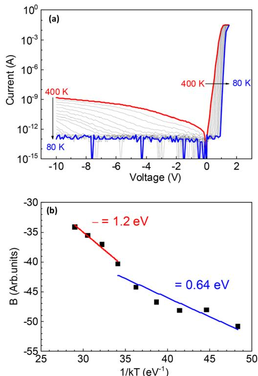
Fig. 5 (a)  $I$ - $V$  characteristics measured at different temperatures after the breakdown for the 380  $\mu\text{m}$  diameter diode; (b) the temperature dependence of coefficient  $B$  in Poole-Frenkel equation, used to calculate the height of the barrier  $\phi$ .
