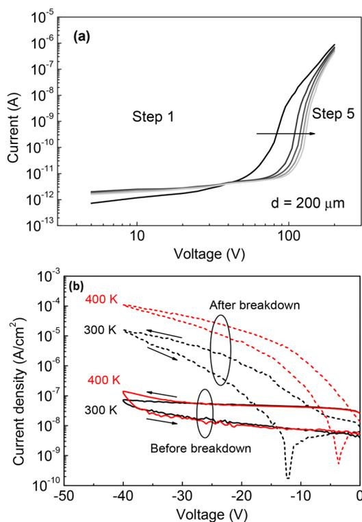
Fig. 8 (a) Current–voltage characteristics measured on 200  $\mu\text{m}$  diameter diode in several consecutive tries; (b) reverse current hysteresis before (solid lines) and after (dashed lines) breakdown; measurements are shown for 300 K (black lines) and 400 K (red lines), the arrows indicate the direction of the voltage sweep.
