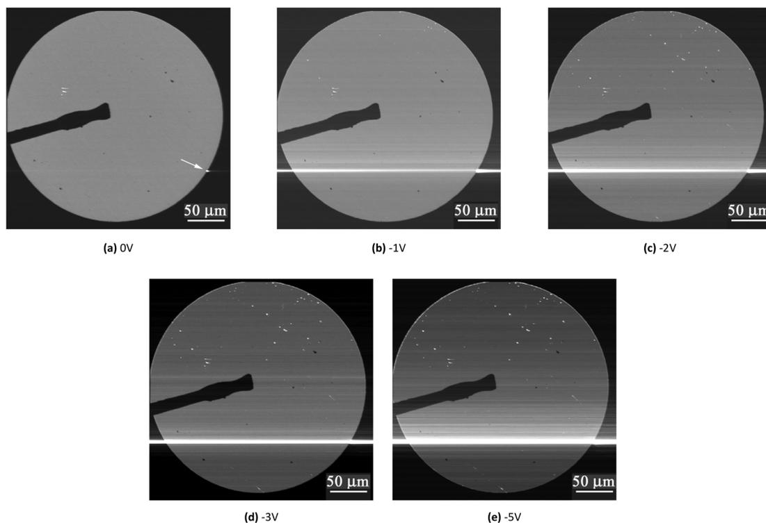
Fig. 7 EBIC maps of the 300  $\mu\text{m}$  diode after breakdown for different applied reverse voltages.
