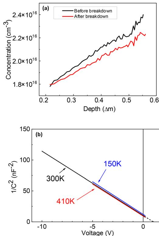
Fig. 3 (a) Room temperature charge concentration profiles calculated from  $C$ - $V$  measurements before breakdown (black line) and after breakdown (red line); (b)  $1/C^2$  versus voltage plots for the 380  $\mu\text{m}$  diameter diode at different temperatures.
