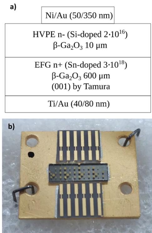
Fig. 1 Ga<sub>2</sub>O<sub>3</sub>-based Schottky diode. (a) – diode structure, (b) – sample photo.
