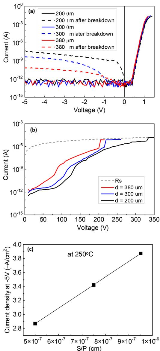
Fig. 2 (a) Room temperature  $I$ - $V$  characteristics measured for diode diameters 200, 300 and 380  $\mu\text{m}$  before and after electric breakdown; (b) reverse current voltage characteristics at high voltages for different diode diameters, the dashed line shows the current limited by the 20 M $\Omega$  resistor in series; (c) current density at 250  $^{\circ}\text{C}$  at -5 V as a function of the ratio of diodes area  $S$  to diodes perimeter  $P$ .
