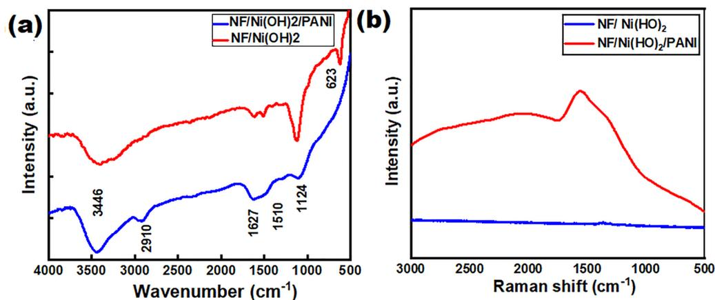
Fig. 2 (a) FT-IR spectrum of NF/Ni(OH)<sub>2</sub>/PANI and (b) Raman spectrum of NF/Ni(OH)<sub>2</sub>/PANI.
