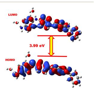
Fig. 7 Frontier orbitals of PANI and PANI-H<sub>3</sub>O<sup>+</sup> at the DFT B3LYP/6-311G+(d,p) level of theory
