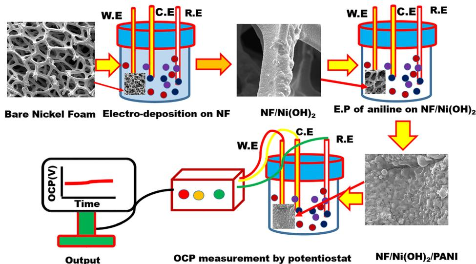
Scheme 1 Modification process of NF/Ni(OH)<sub>2</sub>/PANI and its application to determine pH.
