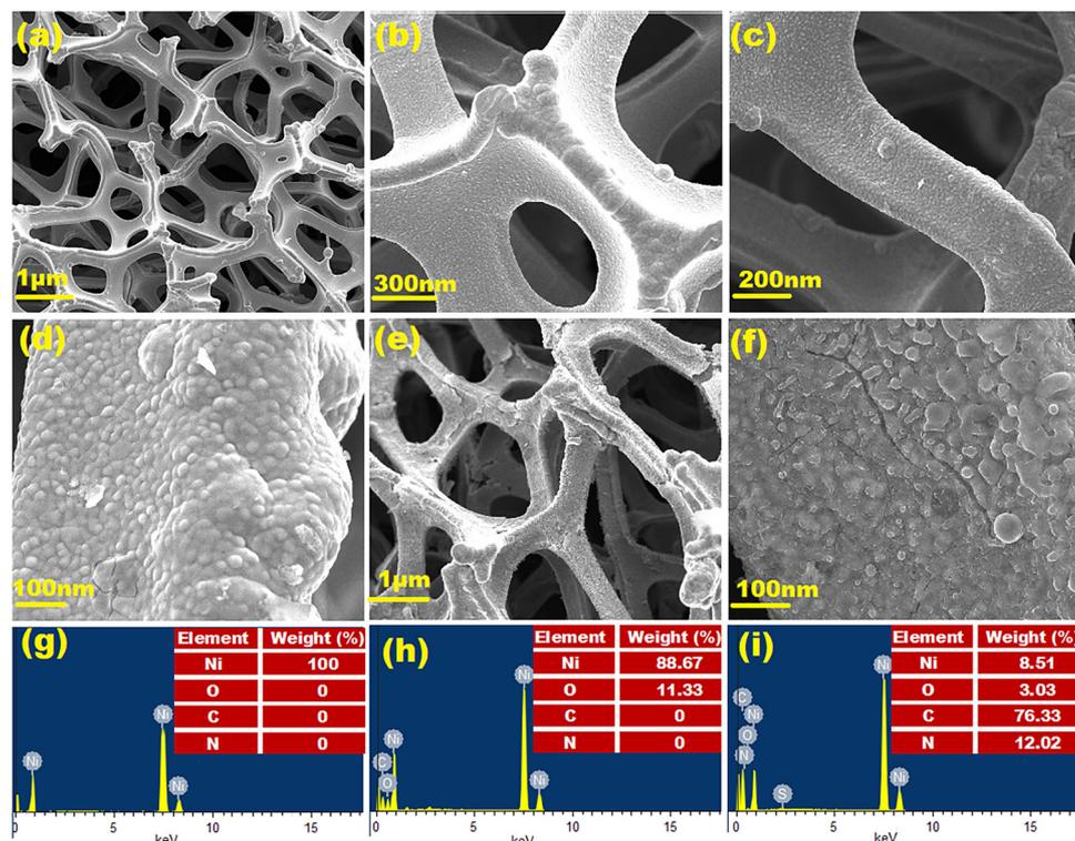
Fig. 1 FESEM images of (a) and (b) NF, (c) and (d) NF/Ni(OH)<sub>2</sub>, (e) and (f) NF/Ni(OH)<sub>2</sub>/PANI and EDAX spectrum of (g) NF, (h) NF/Ni(OH)<sub>2</sub> and (i) NF/Ni(OH)<sub>2</sub>/PANI, respectively.
