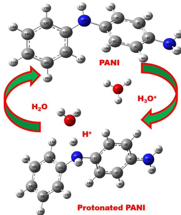
Fig. 6 Sensing mechanism analysis at the DFT B3LYP/6-311G+(d,p) level of theory.
