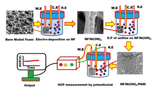
Scheme 1 Modification process of NF/Ni(OH)<sub>2</sub>/PANI and its application to determine pH.
