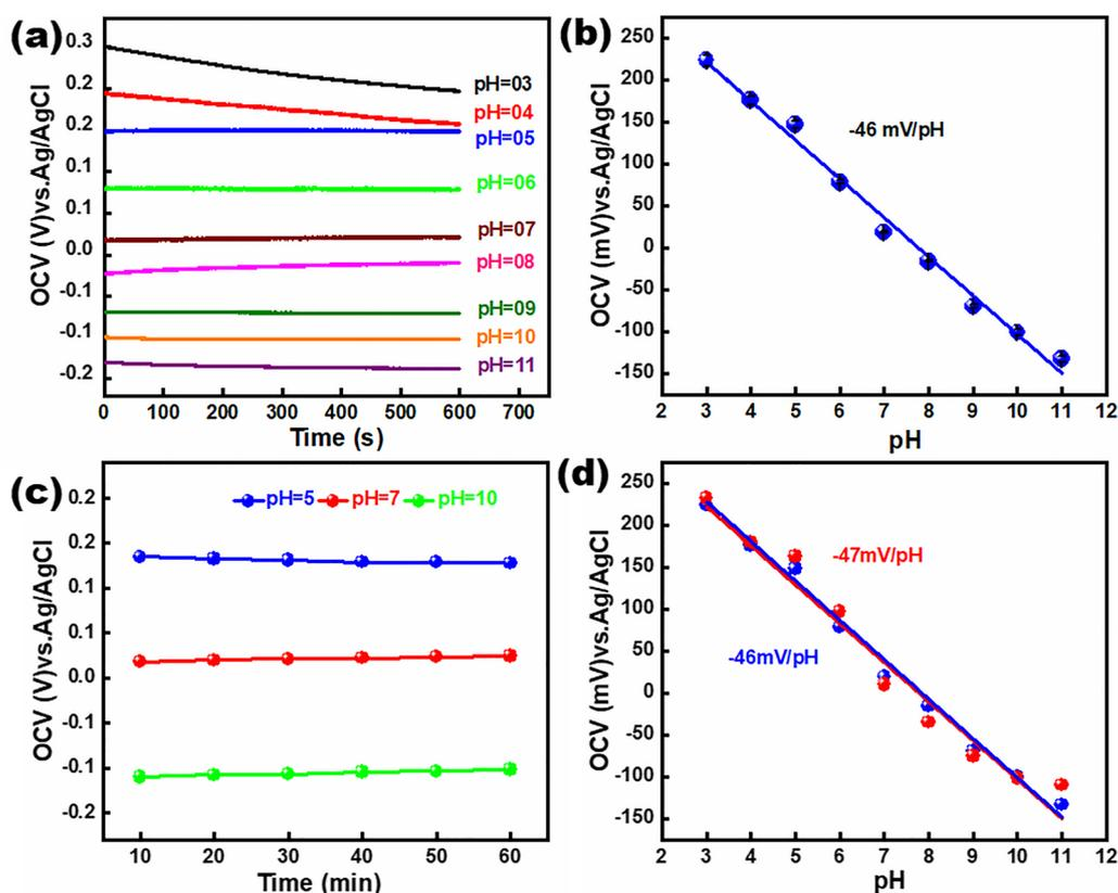
Fig. 4 (a) Potential response of NF/Ni(OH)<sub>2</sub>/PANI at different pH values (3–11) in 0.1 M buffer solution, and (b) the corresponding linear relation plot of pH (3–11), (c) reproducibility, and (d) potential drift measurements.
