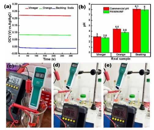
Fig. 5 OCV of the real sample test of vinegar, orange, and baking powder and (b) comparison of an NF/Ni(OH)<sub>2</sub>/PANI pH sensor with the commercial pH sensor. Image of the real sample test (d) vinegar, (e) orange and (f) baking powder.
