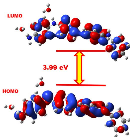
**Fig. 7** Frontier orbitals of PANI and PANI-H<sub>3</sub>O<sup>+</sup> at the DFT B3LYP/6-311G+(d,p) level of theory.
