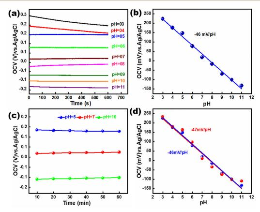
Fig. 4 (a) Potential response of NF/Ni(OH) $_2$ /PANI at different pH values (3–11) in 0.1 M buffer solution, and (b) the corresponding linear relation plot of pH (3–11), (c) reproducibility, and (d) potential drift measurements.
