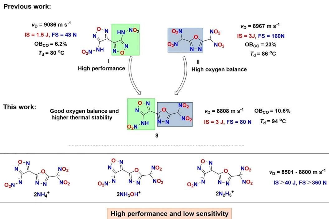
Fig. 1 The design of novel energetic compounds.
