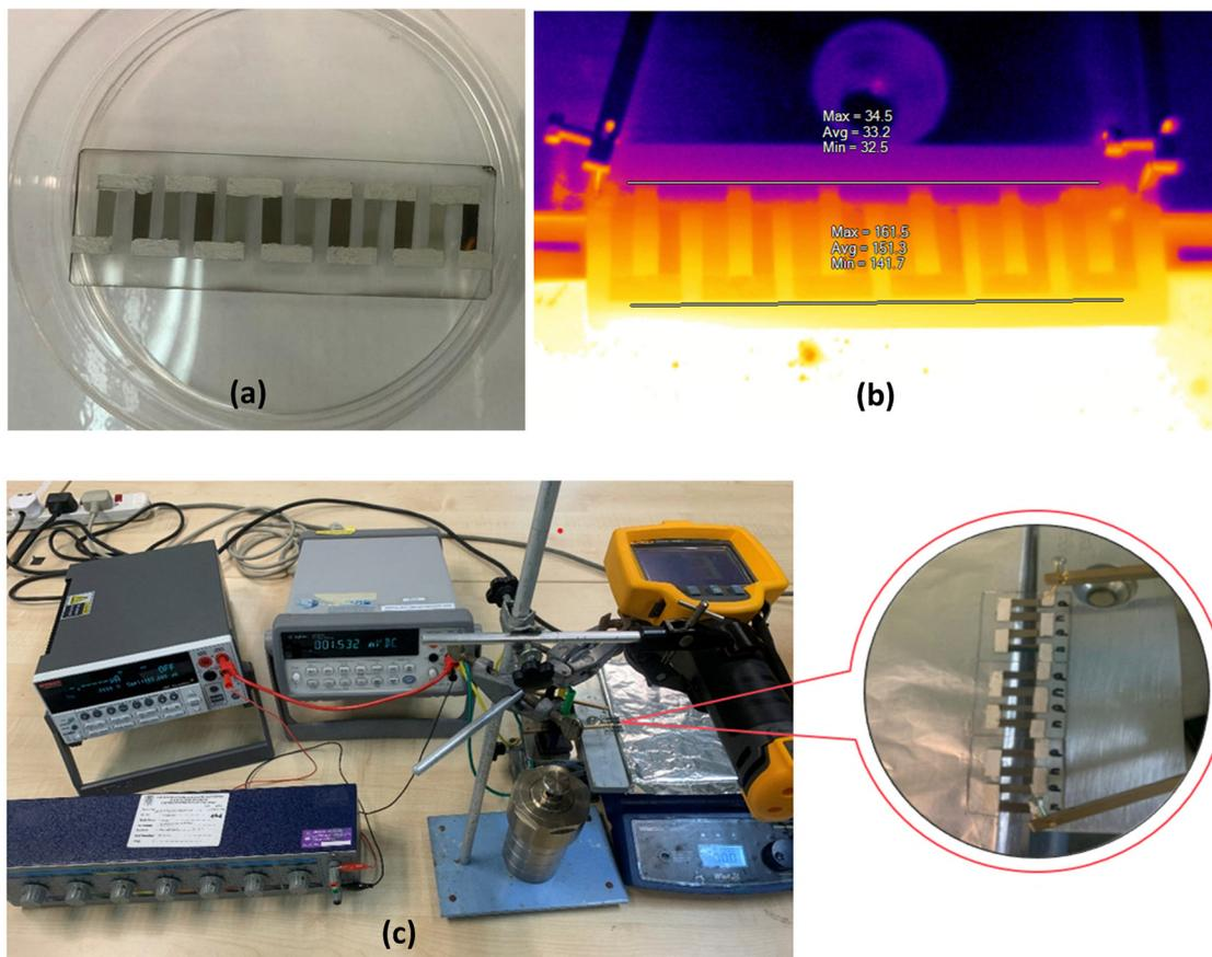
Fig. 2 (a) The fabricated  $\text{Bi}_2\text{Te}_3/\text{Sb}_2\text{Te}_3$  thin film TEG. (b) Thermal image of a  $\text{Bi}_2\text{Te}_3/\text{Sb}_2\text{Te}_3$  thin film TEG in operation. (c) Picture of the custom IVP measurement setup.
