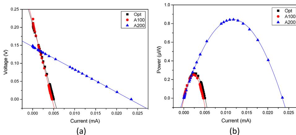
Fig. 8 (a)  $IV$  and (b)  $IP$  plots of the optimized  $\text{Bi}_2\text{Te}_3/\text{Sb}_2\text{Te}_3$  thin film TEG, annealed at 100 and 200 °C.
