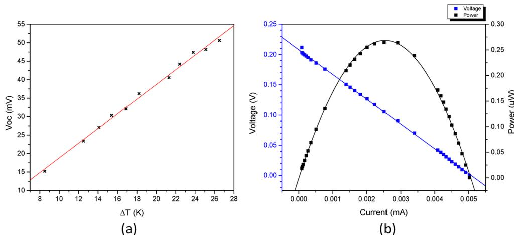
Fig. 7 (a)  $V_{oc}$  vs.  $\Delta T$  and (b) IVP plot of the optimized  $\text{Bi}_2\text{Te}_3/\text{Sb}_2\text{Te}_3$  thin film TEG.
