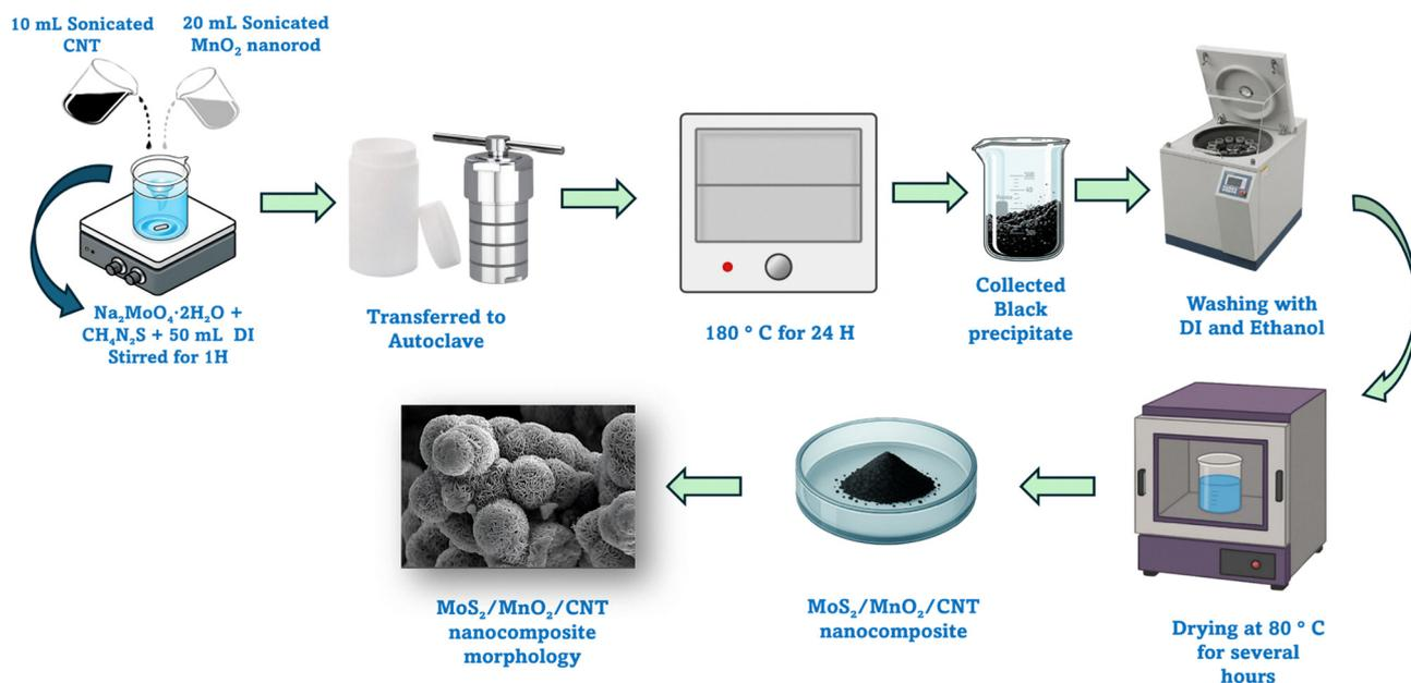
Fig. 1 Schematic diagram of the synthesis of the MoS<sub>2</sub>/MnO<sub>2</sub>/CNT composite through a hydrothermal route.
