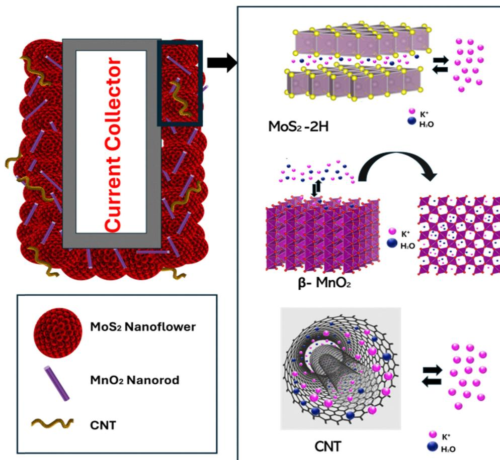
**Fig. 12** Schematic of K<sup>+</sup> ion and H<sub>2</sub>O insertion and extraction from the electrolyte into the MoS<sub>2</sub>/MnO<sub>2</sub>/CNT composite electrode.
