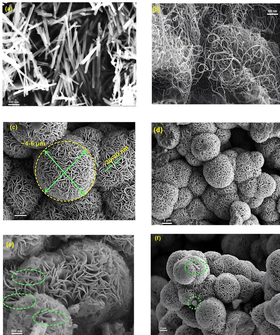
Fig. 4 (a) and (b) SEM images of MnO<sub>2</sub> nanorods and CNTs, respectively; (c)–(f) SEM images of the MoS<sub>2</sub> nanoflower, MoS<sub>2</sub>/MnO<sub>2</sub> (3 wt%), MoS<sub>2</sub>/MnO<sub>2</sub> (5 wt%) and MoS<sub>2</sub>/MnO<sub>2</sub> (5 wt%)/CNT (1 wt%) nanocomposites, respectively.
