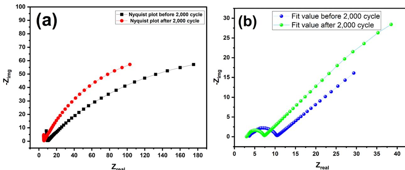
Fig. 8 Nyquist plots of the MoS<sub>2</sub>/MnO<sub>2</sub> (5 wt%)/CNT (1 wt%) nanocomposite (a) before and after 2000 cycles of charging–discharging and (b) fitted before and after 2000 cycles of charging–discharging.
