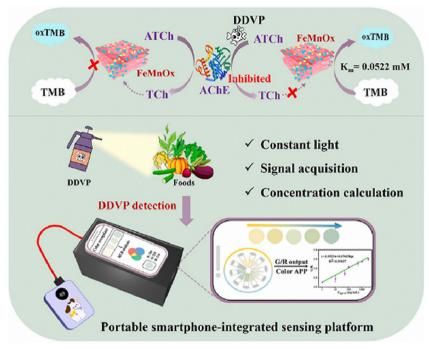
Fig. 5 Illustration of a smartphone-integrated portable colorimetric detection platform using FeMnO<sub>x</sub> nanozyme for quantifying DDVP (Licensed under ref 124)
