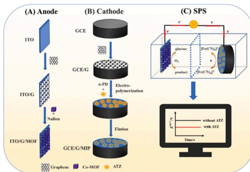
Fig. 6 The process involves preparing the MOF- customized anode (A), cathode (B), setup and detection steps for self-powered (C) (Licensed under ref. 144).
