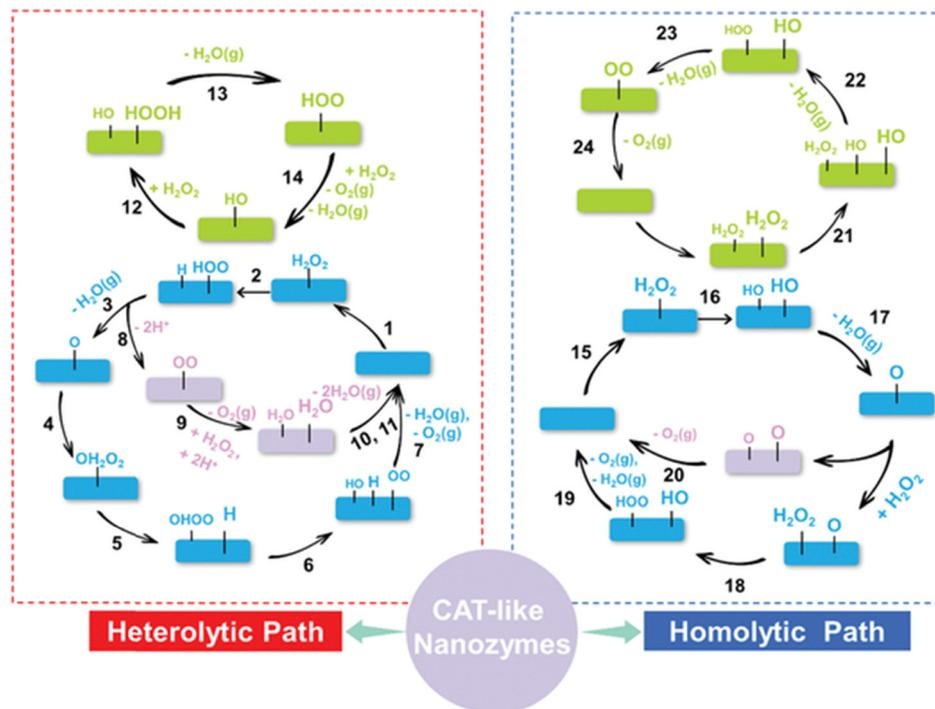
Fig. 2 Schematic representation of the catalytic mechanism of CAT-like nanozymes; the single ring on the left denotes the heterolytic reaction pathway, whereas the double ring on the right corresponds to the homolytic pathway (Licensed under ref. 86).
