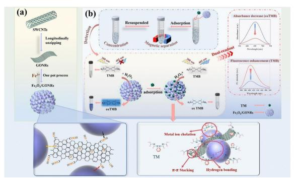
Fig. 7 (a) The synthesis procedure of  $Fe_3O_4/GONRs$  (b) schematic representation of the dual-mode detection of TM using fluorescence and colorimetric methods (Licensed under ref. 164).
