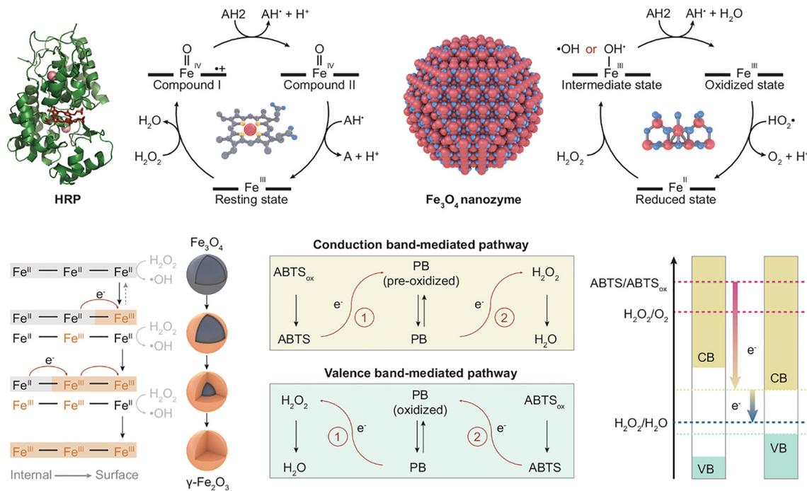
Fig. 1 A schematic illustration showing the relationship between nanozyme morphology and catalytic performance<sup>75</sup> [Licensed under a Creative Commons Attribution-NonCommercial-NoDerivatives 4.0 International License].
