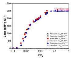
Fig. 5 Volumetric N<sub>2</sub> adsorption isotherms at 77 K for ZIF-8<sup>mono</sup> and Ni-, Co- and Cu-doped variants
