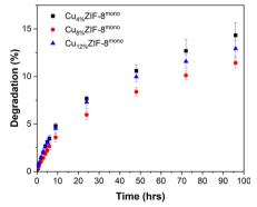
Fig. 7 Time-dependent degradation of ZIF-8<sup>mono</sup> and its doped variants during RhB adsorption in aqueous solution.
