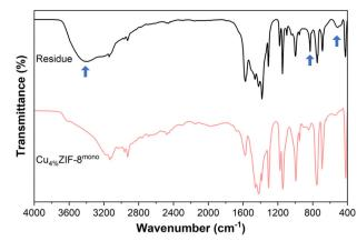
Fig. 8 FTIR spectra of the as-synthesised  $Cu_{4\%}$ ZIF-8<sup>mono</sup> and its white residue obtained following the stability test. The blue arrows indicate the appearance of new peaks.
