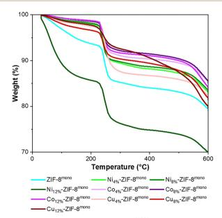
Fig. 4 Thermogravimetric analysis of ZIF-8<sup>mono</sup> and its doped variants.
