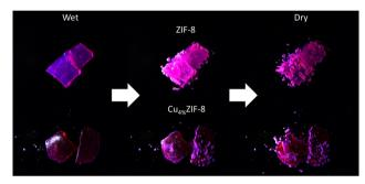
Fig. 9 Optical images of the peeling process during the drying of ZIF-8mono and  $Cu_{4\%}$ ZIF-8<sup>mono</sup> following the RhB adsorption test.
