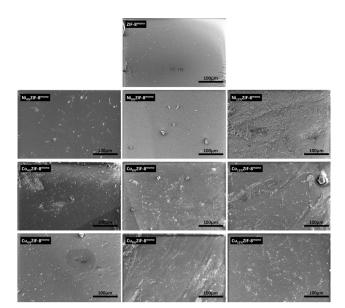
Fig. 3 SEM images of ZIF-8<sup>mono</sup> and its Ni-, Co- and Cu-doped variants.
