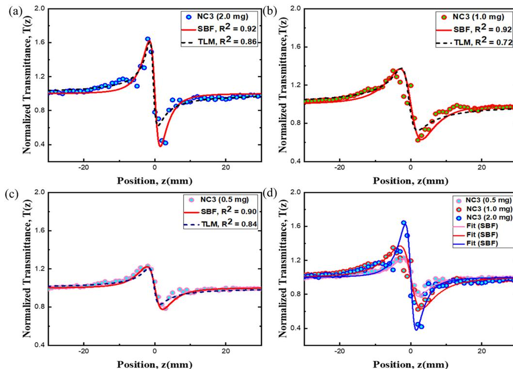
Fig. 13 CA Z-scan experimental data with the theoretical fit of NC3 [SnO<sub>2</sub>-rGO (2.5:1)] nanocomposites (a) NC3 (2.0 mg ml<sup>-1</sup>), (b) NC3 (1.0 mg ml<sup>-1</sup>) and (c) NC3 (0.5 mg ml<sup>-1</sup>), respectively, at a peak intensity of  $I_0 = 5.3 \text{ kW cm}^{-2}$ . (d) Peak-valley difference in a single plot.
