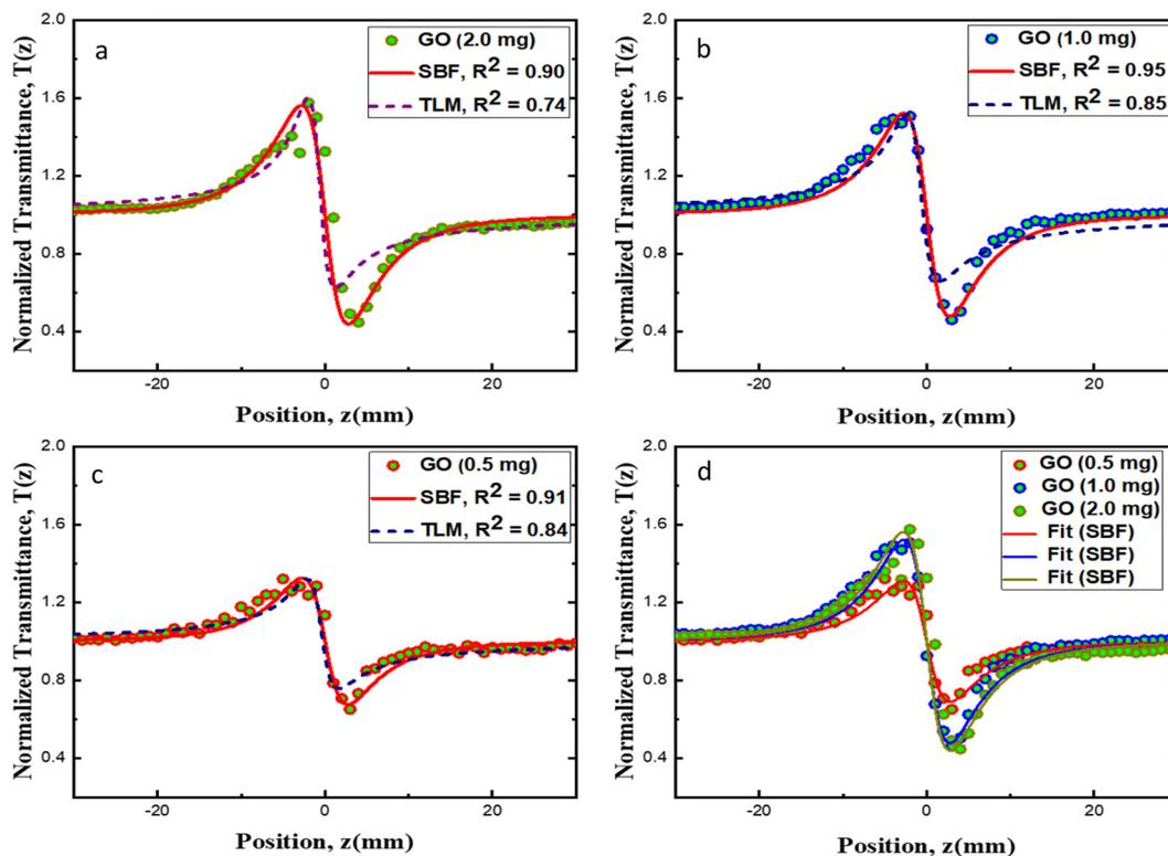
Fig. 9 CA Z-scan experimental data with the theoretical fit of GO (a) GO (2.0 mg ml<sup>-1</sup>), (b) GO (1.0 mg ml<sup>-1</sup>), and (c) GO (0.5 mg ml<sup>-1</sup>), respectively, at a peak intensity of  $I_0 = 5.3 \text{ kW cm}^{-2}$ . (d) Peak-valley difference in a single plot.
