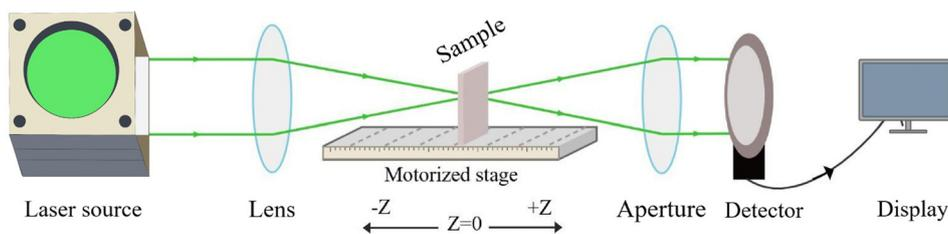
Fig. 2 Schematic diagram of the Z-scan setup.
