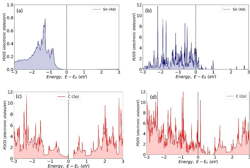
Fig. 16 PDOS plot for the Sn 4d orbital of SnO<sub>2</sub>, (a) before and (b) after forming a heterostructure with rGO. PDOS plot for the C 2p orbital of rGO, (c) before and (d) after forming a heterostructure with SnO<sub>2</sub>.
