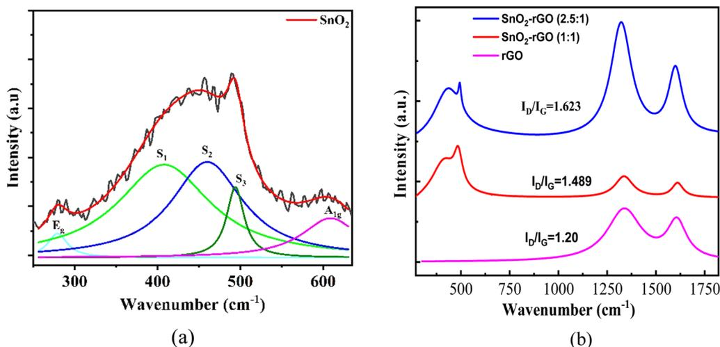
Fig. 6 (a) Raman spectra of the synthesized  $\text{SnO}_2$ , and (b) Raman spectra of the synthesized rGO, and  $\text{SnO}_2$ -rGO nanocomposites.
