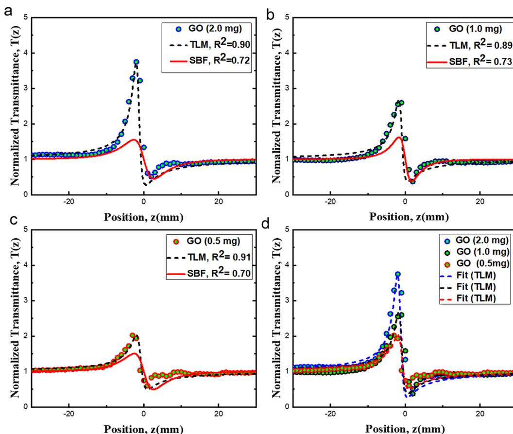
Fig. 8 CA Z-scan experimental data with the theoretical fit of GO nano-composites (a) GO (2.0 mg ml<sup>-1</sup>), (b) GO (1.0 mg ml<sup>-1</sup>), and (c) GO (0.5 mg ml<sup>-1</sup>), respectively, at a peak intensity of  $I_0 = 1.00$  kW cm<sup>-2</sup>. (d) Peak-valley difference in a single plot.
