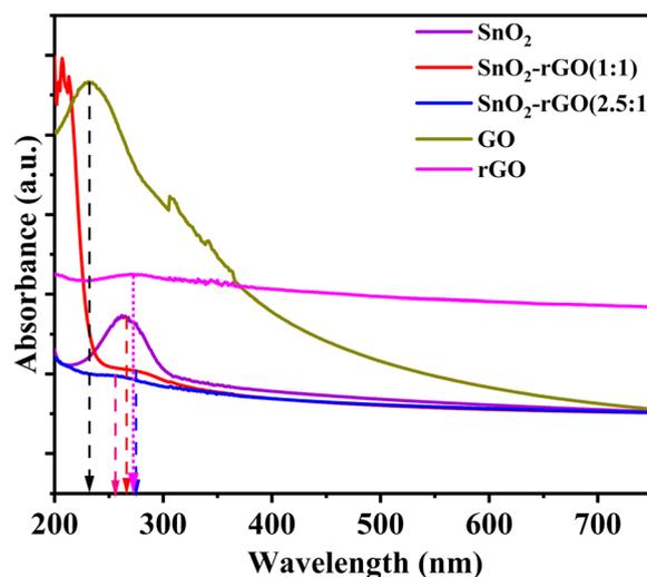
Fig. 3 Exploring optical properties of SnO<sub>2</sub>, GO, rGO, and SnO<sub>2</sub>-rGO nanocomposites through UV-vis spectroscopy.
