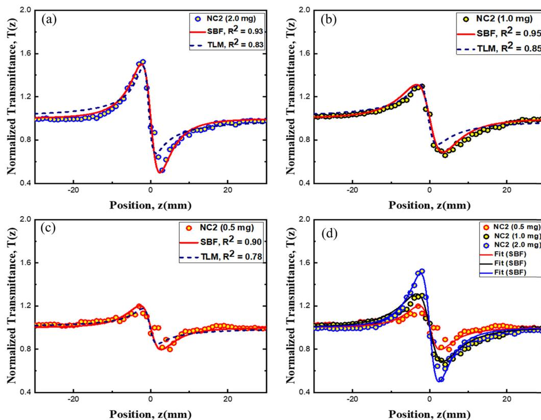
Fig. 12 CA Z-scan experimental data with the theoretical fit of NC2 [SnO<sub>2</sub>-rGO (1.25 : 1)] nanocomposites (a) NC2 (2.0 mg ml<sup>-1</sup>), (b) NC2 (1.0 mg ml<sup>-1</sup>) and (c) NC2 (0.5 mg ml<sup>-1</sup>), respectively, at a peak intensity of  $I_0 = 5.3 \text{ kW cm}^{-2}$ . (d) Peak-valley difference in a single plot.
