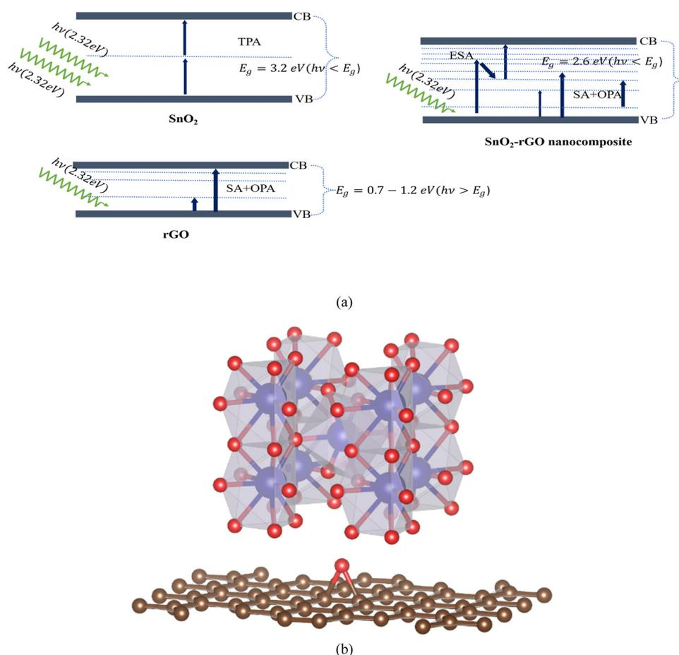
Fig. 15 (a) Schematic energy diagram for the NA and SA mechanisms, and (b) optimized structure of the SnO<sub>2</sub>-rGO heterostructure. Red, brown, and blue colored atoms represent O, C, and Sn, respectively.
