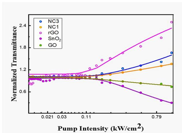
Fig. 17 Normalized transmittance as functions of pump intensity for SnO<sub>2</sub>, GO, rGO, and SnO<sub>2</sub>-rGO nanocomposites under an intensity of 1.00 kW cm<sup>-2</sup> (532 nm).
