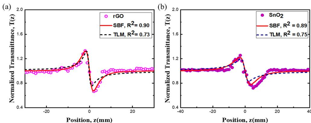
**Fig. 10** CA Z-scan experimental data with the theoretical fit of (a) rGO (2.0 mg ml<sup>-1</sup>) and (b) SnO<sub>2</sub> (2.0 mg ml<sup>-1</sup>) at a peak intensity of  $I_0 = 5.3$  kW cm<sup>-2</sup>.
