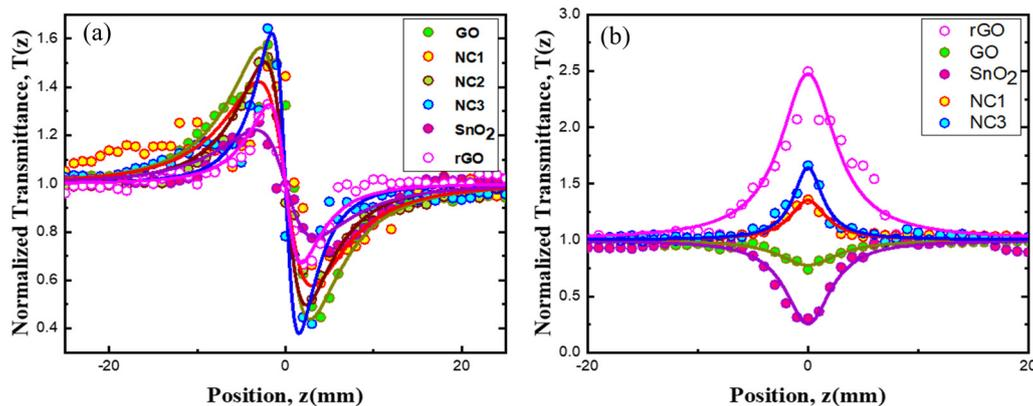
Fig. 14 (a) Normalized close-aperture (CA) data with theoretical fitting in a single plot for pure SnO<sub>2</sub>, GO, rGO, NC1, NC2, and NC3 nanocomposites with different mass ratios of maximum concentrations (2.0 mg ml<sup>-1</sup>) at  $I_0 = 5.3 \text{ kW cm}^{-2}$ . (b) Normalized open-aperture (OA) data with theoretical fitting in a single plot for pure SnO<sub>2</sub>, GO, rGO, NC1, and NC3 of two different ratios at  $I_0 = 1.00 \text{ kW cm}^{-2}$ .
