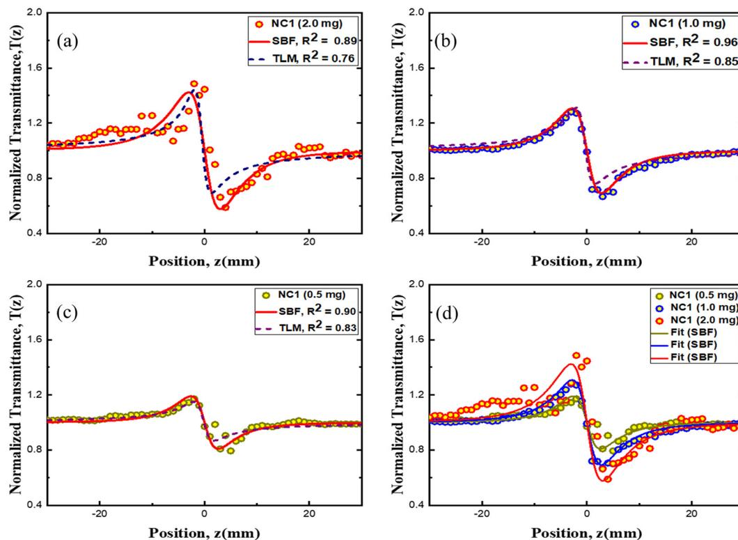
Fig. 11 CA Z-scan experimental data with the theoretical fit of NC1 [SnO<sub>2</sub>-rGO (1 : 1)] nanocomposites (a) NC1 (2.0 mg ml<sup>-1</sup>), (b) NC1 (1.0 mg ml<sup>-1</sup>) and (c) NC1 (0.5 mg ml<sup>-1</sup>) respectively at a peak intensity of  $I_0 = 5.3 \text{ kW cm}^{-2}$ . (d) Peak-valley difference in a single plot.
