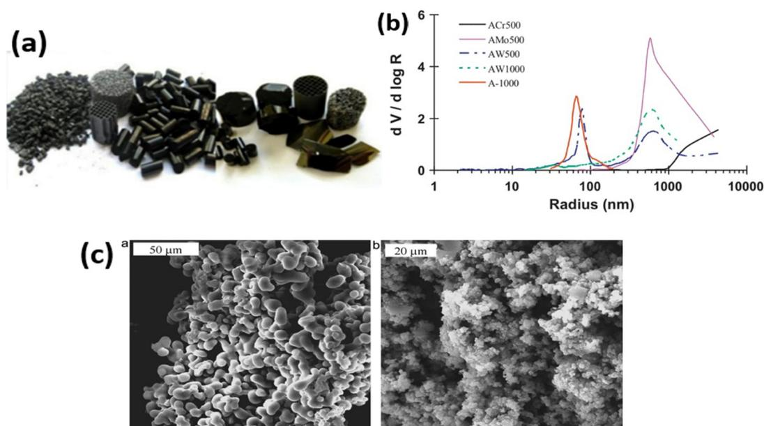
**Fig. 22** (a) Carbon gels formed in various shapes. (b) Pore size distribution of metal-doped carbon aerogels *via* mercury porosimetry. (c) SEM images revealing surface morphology of ACr500 and AW500 samples. Reproduced from ref. 278 and 279 with permission from Elsevier, copyright 2013 and 2011.
