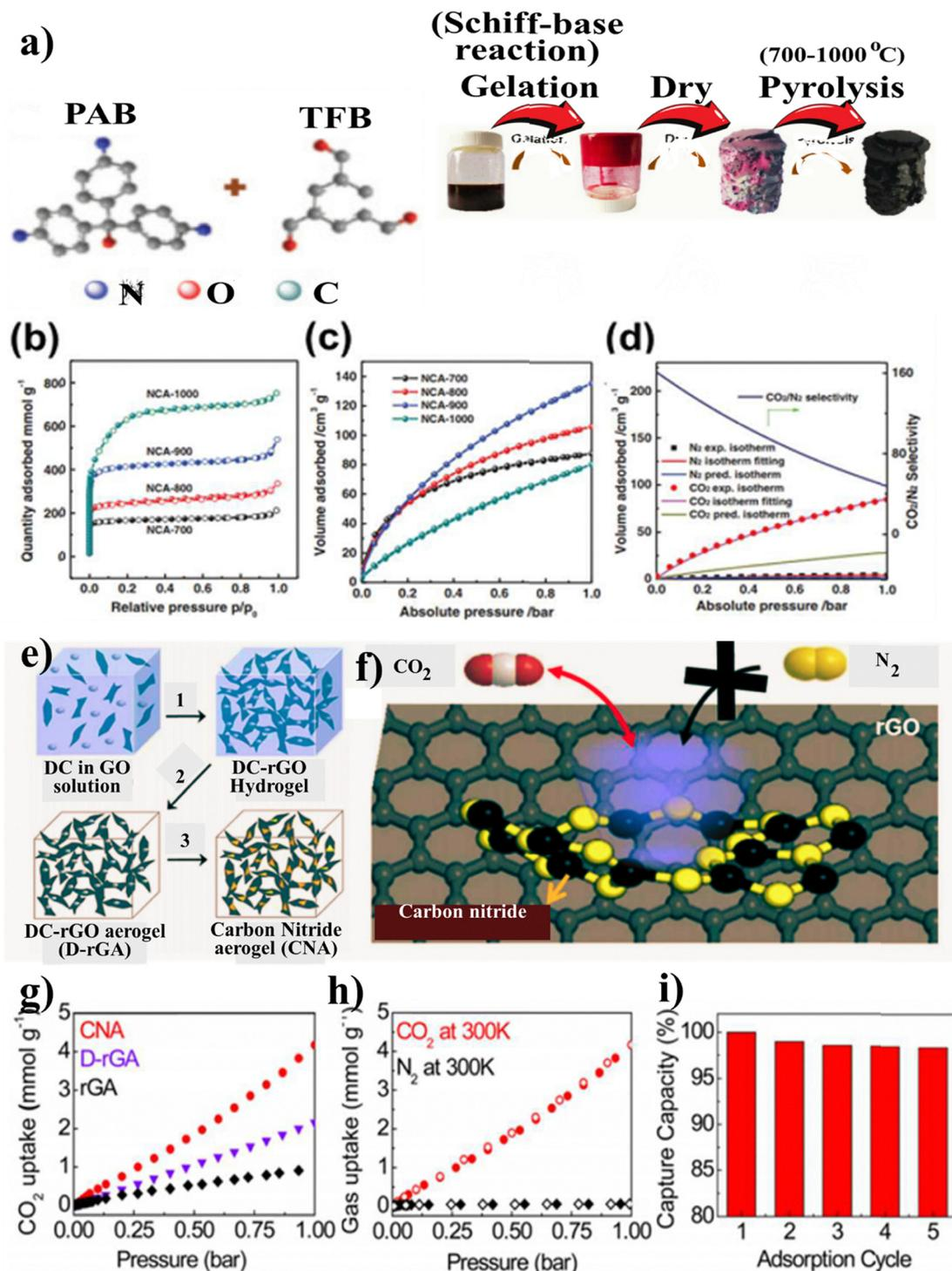
Fig. 20 (a) and (b) Synthesis and  $N_2$  sorption isotherms of nitrogen-doped carbon aerogels (NCAs). (c) and (d)  $CO_2$  uptake and  $CO_2/N_2$  selectivity of NCAs. (e) and (f) Synthesis of the carbon nitride aerogel (CNA) and mechanism of selective  $CO_2$  adsorption. (g)–(i)  $CO_2/N_2$  adsorption behavior and recyclability of CNA. Reproduced from ref. 205 with permission from Elsevier, copyright 2020.
