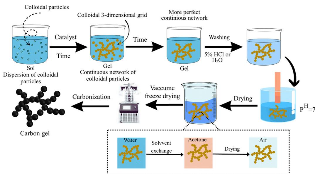
Fig. 7 Process flow for carbon gel synthesis.
