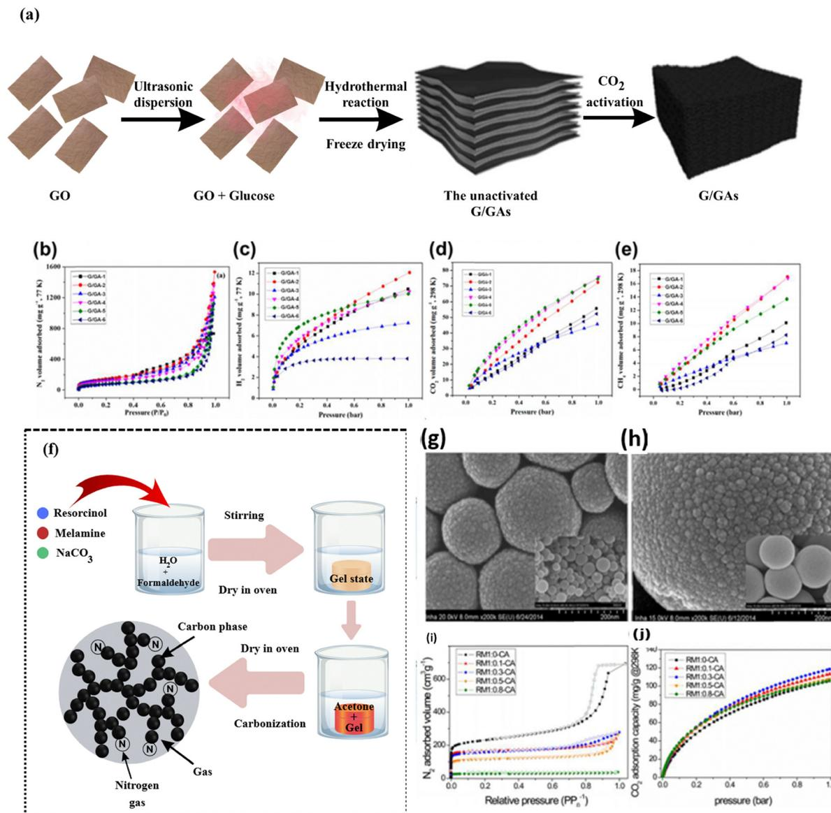
Fig. 21 (a) Synthesis of 3D glucose/graphene aerogels (G/GAs). (b)–(e) Gas adsorption behavior of G/GAs for  $N_2$ ,  $H_2$ ,  $CO_2$ , and  $CH_4$ . (f)–(h) Fabrication and SEM analysis of nitrogen-doped carbon aerogels, with adsorption profiles influenced by precursor ratios. (i), (j)  $N_2$  adsorption–desorption isotherms and pore size distribution curves of nitrogen-doped carbon aerogels, respectively. Reproduced from ref. 205 with permission from Elsevier, copyright 2020.
