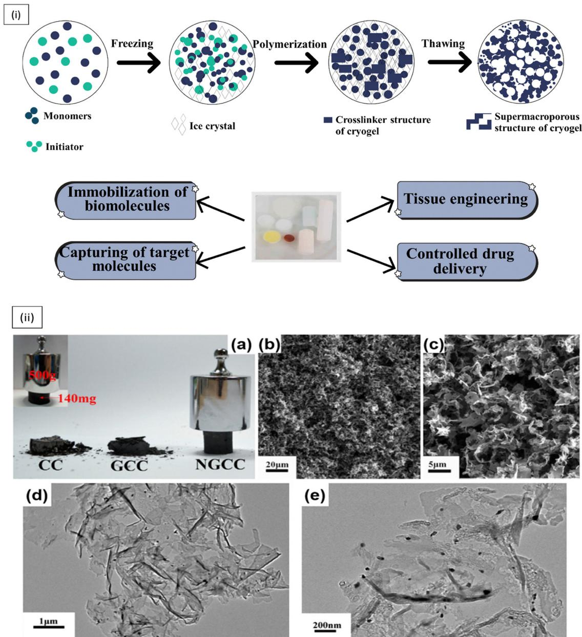
**Fig. 5** (i) Schematic of the cryogel formation process. (ii) (a) Photographs of the carbon cryogel (CC), graphene/carbon cryogel (GCC), and Ni-doped graphene/carbon cryogel (NGCC), each weighing 90 mg, supporting a 200 g load (inset: a 140 mg NGCC monolith supporting a 500 g weight). (b) and (c) SEM images and (d) and (e) TEM images of the Ni-doped graphene/carbon cryogel are also shown. Reproduced from ref. 75 and 80 with permission from Elsevier & ACS, copyright 2023 & 2013.
