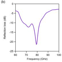
Fig. 6 (a) Photograph of the fabricated millimeter-wave-absorbing film on a metal plate. (b) Observed *RL* spectrum of the film.
