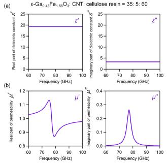
Fig. 4 Frequency dependence of (a)  $\epsilon'$  and  $\epsilon''$ , (b)  $\mu'$  and  $\mu''$  for the composite ( $\epsilon$ -Ga<sub>0.45</sub>Fe<sub>1.55</sub>O<sub>3</sub>:CNT:cellulose resin = 35:5:60) evaluated from the absorption spectrum of the sheet-form sample.
