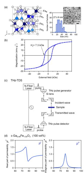
**Fig. 1** (a) Crystal structure, TEM image, particle size distribution of ε-Ga<sub>0.45</sub>Fe<sub>1.55</sub>O<sub>3</sub> nanomagnets. (b) Magnetization *versus* external magnetic field curve of ε-Ga<sub>0.45</sub>Fe<sub>1.55</sub>O<sub>3</sub> measured at 300 K. (c) Diagram of the THz-TDS system. (d) Frequency dependence of  $\mu'$  and  $\mu''$  for ε-Ga<sub>0.45</sub>Fe<sub>1.55</sub>O<sub>3</sub> nanomagnets, calibrated by the filling ratio.
