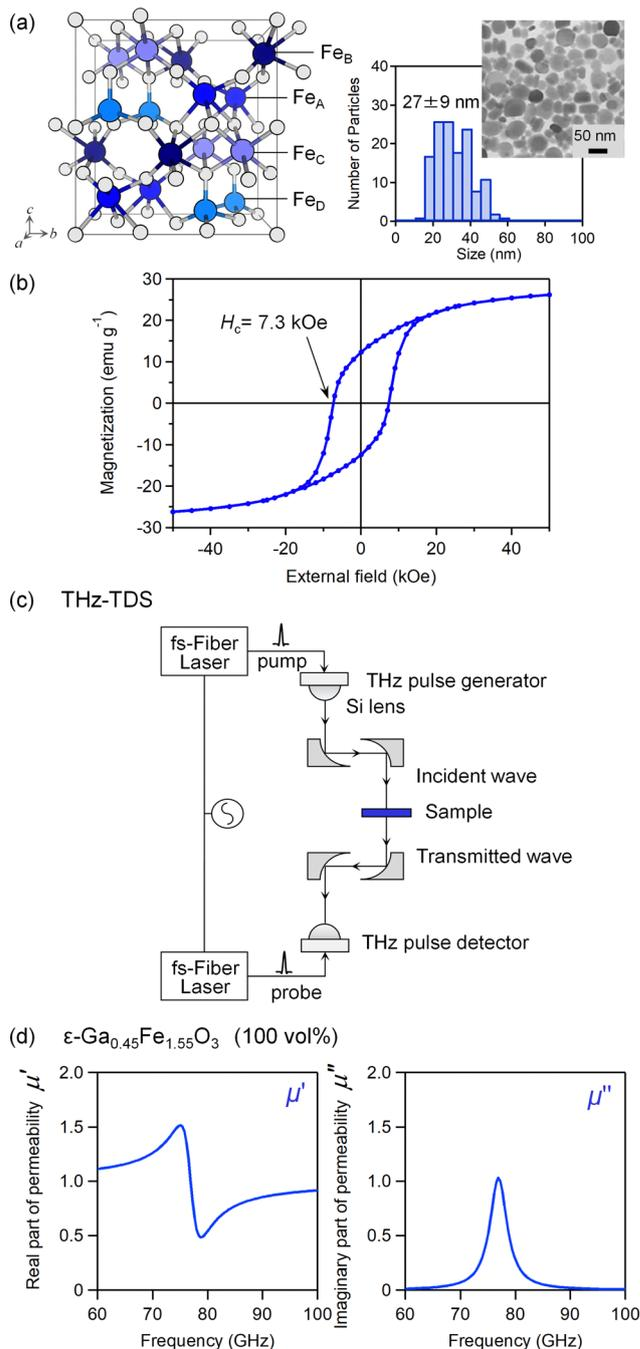
Fig. 1 (a) Crystal structure, TEM image, particle size distribution of  $\epsilon\text{-Ga}_{0.45}\text{Fe}_{1.55}\text{O}_3$  nanomagnets. (b) Magnetization versus external magnetic field curve of  $\epsilon\text{-Ga}_{0.45}\text{Fe}_{1.55}\text{O}_3$  measured at 300 K. (c) Diagram of the THz-TDS system. (d) Frequency dependence of  $\mu'$  and  $\mu''$  for  $\epsilon\text{-Ga}_{0.45}\text{Fe}_{1.55}\text{O}_3$  nanomagnets, calibrated by the filling ratio.
