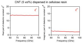
Fig. 3 Frequency dependence of  $\varepsilon'$  and  $\varepsilon''$  for CNTs dispersed in cellulose resin with a concentration of 5 vol%.
