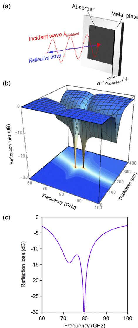
Fig. 5 (a) Schematic illustration of an absorber attached on a metal plate. (b) Three-dimensional map of the simulated  $RL$  value for the composite with respect to the thickness  $d$  and frequency  $f$ . (c) Frequency dependence of the  $RL$  value for an absorber with a thickness of  $231 \mu\text{m}$ , which is an impedance matching condition at  $79 \text{ GHz}$ .
