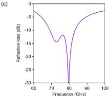
Fig. 5 (a) Schematic illustration of an absorber attached on a metal plate. (b) Three-dimensional map of the simulated RL value for the composite with respect to the thickness d and frequency f. (c) Frequency dependence of the RL value for an absorber with a thickness of 231  $\mu$ m, which is an impedance matching condition at 79 GHz.
