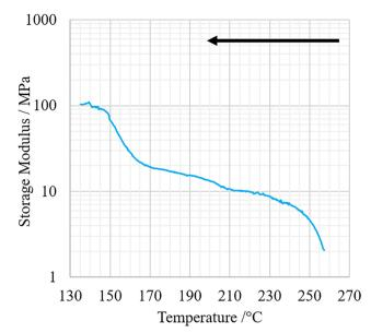
Fig. 4 DMA results for PAEK AM200 from 135-260 °C.
