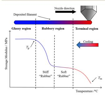
Fig. 1 Standard thermal transitions of polymers
