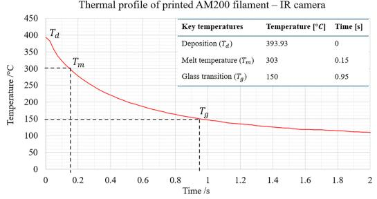
Infrared cooling curve of MEX extruded PAEK AM 200 filament.
