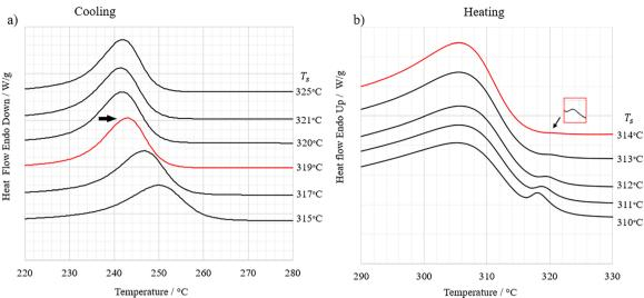
Fig. 6 (a) AM 200 cooling curves at 10  $^{\circ}$ C min $^{-1}$  after 5 min at the indicated  $T_s$ . (b) AM 200 heating curves at 10  $^{\circ}$ C min $^{-1}$  conducted after the cooling curves at 10  $^{\circ}$ C min $^{-1}$ .
