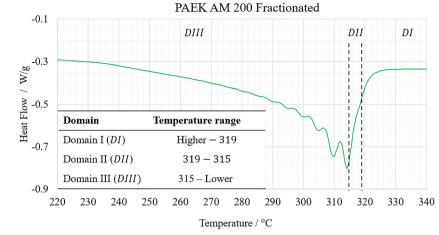
Fig. 7 AM 200 Fractionated DSC curve obtained using a  $T_{\rm s,ideal}$  of 315 °C.
