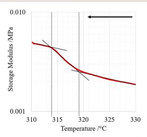
Fig. 3 RR Dynamic temperature ramp conducted on PAEK AM 200 from 310-330 °C
