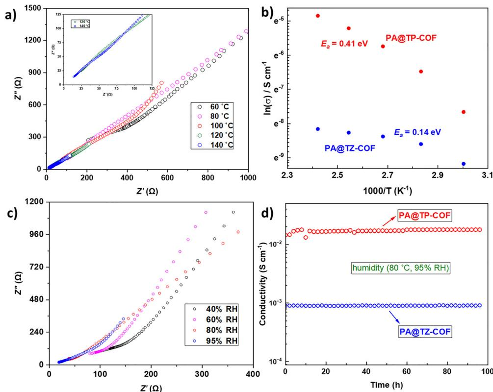
Fig. 3 (a) Nyquist plot for PA@TP-COF under anhydrous conditions. (b) Arrhenius plot for TZ-COF and TP-COF. (c) Nyquist plot for PA@TP-COF under humidified conditions at 80 °C. (d) Stability test carried out by measuring proton conductivity under humidified conditions (80 °C, 95% RH) at an interval of 2 h.
