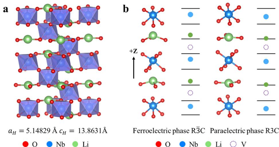
Fig. 2 (a) Ideal structure of LiNbO<sub>3</sub>, (b) ferroelectric phase (left) and paraelectric phase (right) structure of LiNbO<sub>3</sub>.
