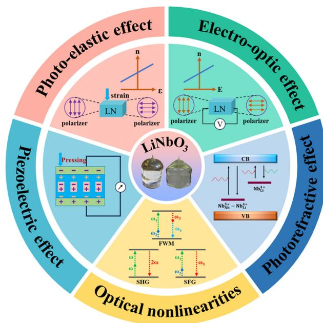
Fig. 1 Properties of LiNbO<sub>3</sub> crystals.
