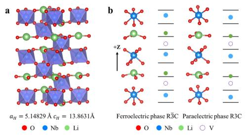
Fig. 2 (a) Ideal structure of LiNbO<sub>3</sub>, (b) ferroelectric phase (left) and paraelectric phase (right) structure of LiNbO<sub>3</sub>.
