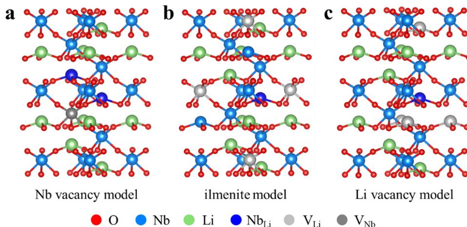
Fig. 3 Defect models in LiNbO<sub>3</sub> crystals. (a) Nb vacancy model, (b) ilmenite model, and (c) Li vacancy model.
