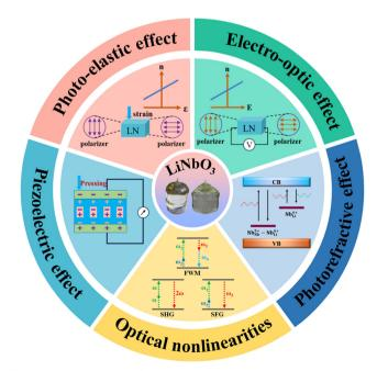
Fig. 1 Properties of LiNbO<sub>3</sub> crystals.
