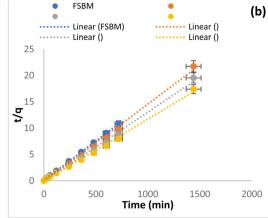
Fig. 8 (a) Adsorption kinetic models, pseudo-first order, (b) pseudo-second-order plots of DR 227 by FSBM, FSBC, ATFSBC, and Cu/FS NCs. The strong alignment with pseudo-second-order kinetics indicates that the adsorption process entails intricate and cooperative supramolecular interactions between the dye and the functional sites on the adsorbent.
