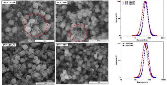
Fig. 8 SEM images and particle size distribution by DLS of the samples with the lowest PVP-0.25/MM, PVP-0.25/MW, and the highest PVP-2/MM and PVP-2/MW molar ratios of PVP synthesized in 6 hours using an ultrasound probe at a constant temperature of 70 °C. Circled red dashed lines are representative of unreacted materials.
