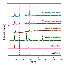
Fig. 2 XRD patterns of MOF samples (PVP-0) synthesized in 2-6 h using an ultrasound probe (70  $^{\circ}$ C). RT = Reaction time. The MOF-235 and MIL-53(Fe) patterns were recorded from CIF files of MOF-235 and MIL-53(Fe).  $^{31,36}$  The unreacted FeCl<sub>3</sub> ( $\bigstar$ ) and H<sub>2</sub>BDC (\*) phases were marked in the patterns. 33,34
