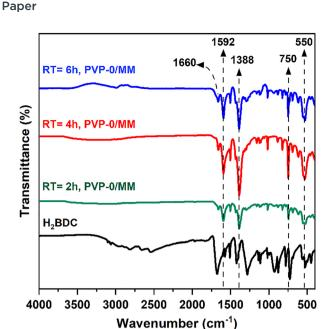
Fig. 1 FTIR spectra of MOF samples (PVP-0) synthesized in 2-6 h using an ultrasound probe at a constant temperature of 70 °C. RT = reaction
