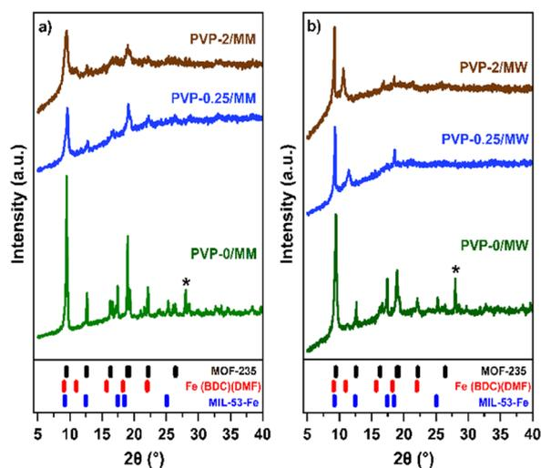
Fig. 7 XRD patterns of MOF samples synthesized in 6 hours under an ultrasound reaction with the lowest (0.25) and the highest (2) molar ratios of PVP at ( $70^\circ\text{C}$ ) and post-synthesis treatment by (a) methanol and (b) methanol–water. Asterisks mark peaks belonging to the  $\text{H}_2\text{BDC}$  phase.<sup>35</sup> The final Rietveld plots were calculated from CIF files of MOF-235 and two different crystal phases of MIL-53(Fe).<sup>31,36,45</sup>
