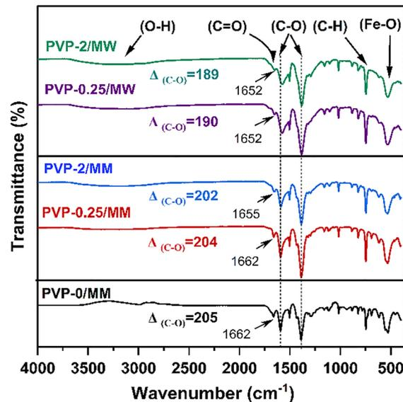
Fig. 6 FTIR spectra of MOF samples synthesized in 6 hours using an ultrasound probe ( $70 \text{ }^\circ\text{C}$ ). Post-synthesis treatment, the lowest (PVP-0.25) and the highest (PVP-2) molar ratios of PVP.  $\Delta$  represents the frequency separation between the symmetric ( $\nu_s$ ) and asymmetric ( $\nu_{as}$ ) vibrations of the carboxyl group.
