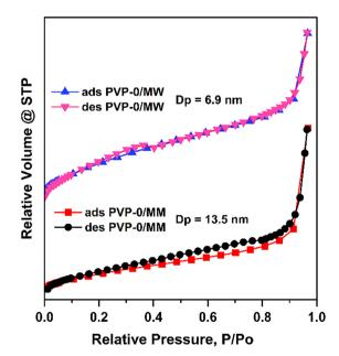
**Fig. 5** Nitrogen adsorption—desorption isotherms,  $(D_{\rm p})$  average pore diameter, as determined using N<sub>2</sub> adsorption—desorption isotherms at 77 K of PVP-0/MM and PVP-0/MW samples synthesized in 6 hours using an ultrasound probe (70 °C).
