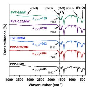
Fig. 6 FTIR spectra of MOF samples synthesized in 6 hours using an ultrasound probe (70 °C). Post-synthesis treatment, the lowest (PVP-0.25) and the highest (PVP-2) molar ratios of PVP.  $\Delta$  represents the frequency separation between the symmetric ( $\nu_s$ ) and asymmetric ( $\nu_{as}$ ) vibrations of the carboxyl group
