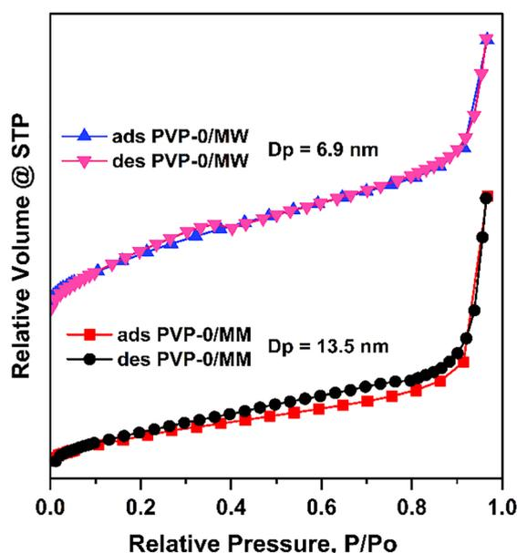
Fig. 5 Nitrogen adsorption–desorption isotherms, ( $D_p$ ) average pore diameter, as determined using  $\text{N}_2$  adsorption–desorption isotherms at 77 K of PVP-0/MM and PVP-0/MW samples synthesized in 6 hours using an ultrasound probe (70 °C).
