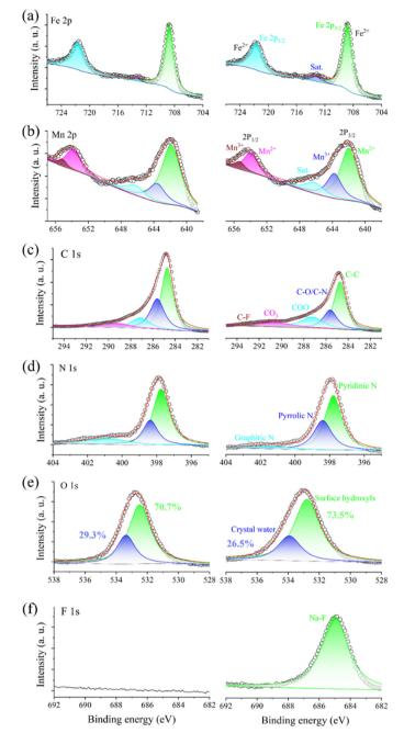
Fig. 7 XPS analysis of the PW/CNT-based cathode in the (a) Fe 2p, (b) Mn 2p, (c) C 1s, (d) N 1s, (e) O 1s, and (f) F 1s before and after activation.
