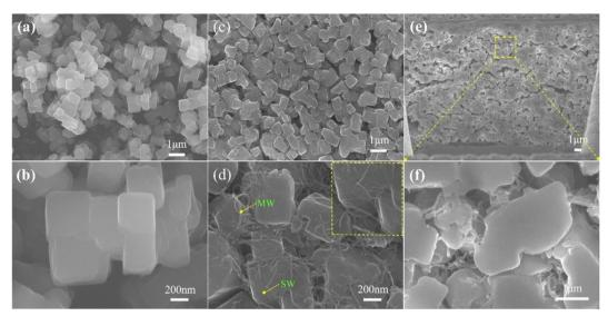
Fig. 2 FE-SEM images of (a) and (b) PW powders, (c) and (d) the PW/CNT electrode surface, and (e) and (f) cross-section.
