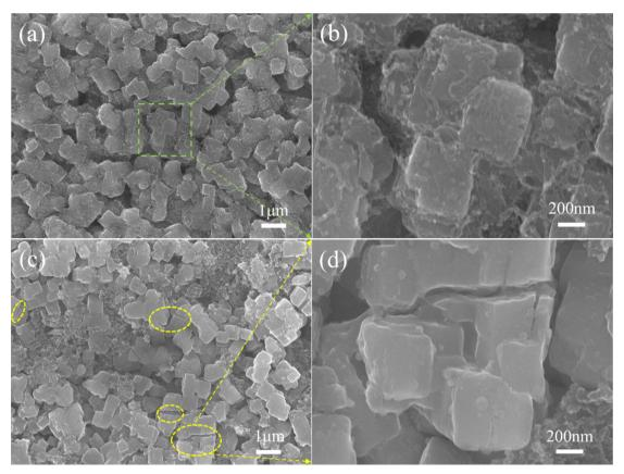
Fig. 5 FE-SEM images of (a) and (b) PW/CNT- and (c) and (d) PW/AB+PVDF-based 150 cycled electrodes.
