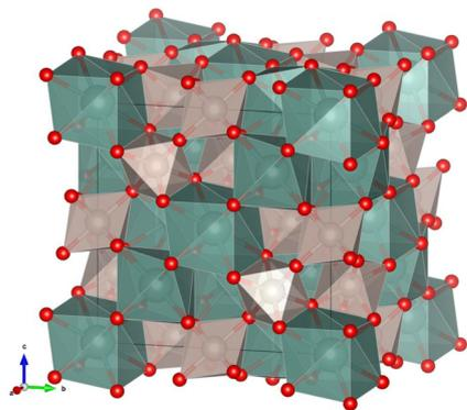
Fig. 2 The pyrochlore unit cell with the teal colour representing Y, the grey colour representing Ru and red representing oxygen.
