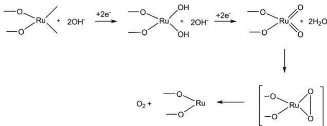
Fig. 8 Proposed cyclic Ru–O intermediate in the OER on ruthenate pyrochlores. Adapted from Horowitz *et al.*<sup>4,63</sup>
