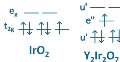
Fig. 14 An illustration of the orbital filling in IrO<sub>2</sub> and Y<sub>2</sub>Ir<sub>2</sub>O<sub>7</sub>.<sup>90</sup>
