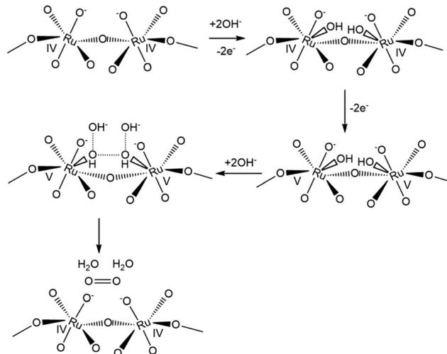
Fig. 10 Detailed OER mechanism with formation of seven-coordinate  $\text{Ru}^{5+}$ . Used with permission of IOP Publishing Limited, from Journal of the Electrochemical Society, Prakash *et al.*<sup>66</sup>, 1948; permission conveyed through Copyright Clearance Center, Inc.
