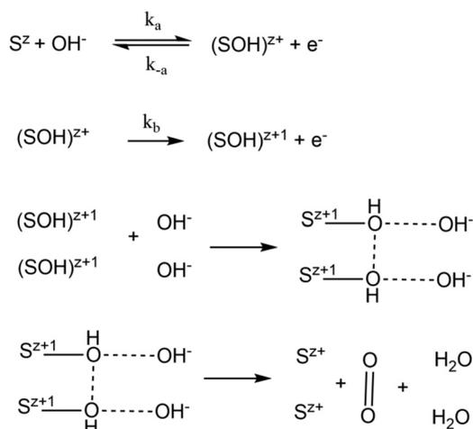
Fig. 9 OER mechanism on Pb–Ru pyrochlore. S denotes an active site.<sup>70</sup>
