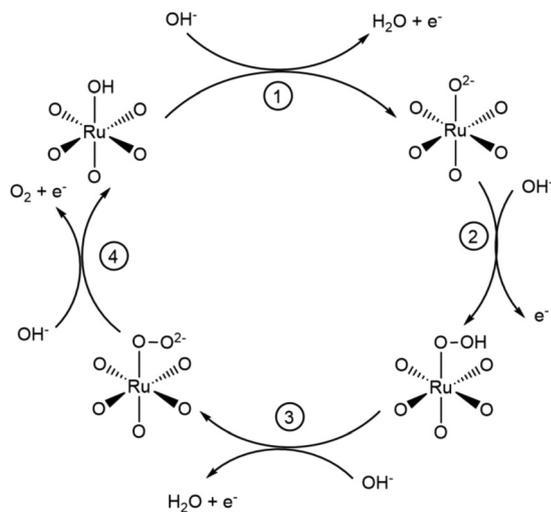
Fig. 11 OER mechanism on lead ruthenate pyrochlores in alkaline media, redrawn with permission from Parrondo *et al.*<sup>72</sup> Copyright Royal Society of Chemistry 2015.
