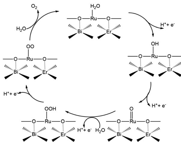
Fig. 12 Illustrated OER pathway in a Bi/Er co-doped pyrochlore. Redrawn from Zhou *et al.*<sup>76</sup>
