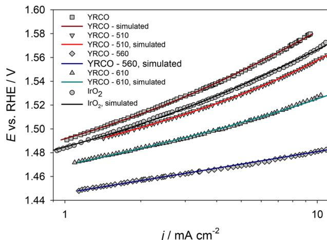
Fig. 16 The CCC equation<sup>143</sup> (eqn 37) fitted to values of electrode potential vs. logarithm of current density for YRCO, YRCO-X, and IrO<sub>x</sub> from Kim *et al.* 2019.<sup>94,143</sup>
