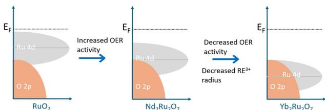
Fig. 13 A schematic illustration of the rigid band structures for RuO<sub>2</sub>, Yb<sub>2</sub>Ru<sub>2</sub>O<sub>7</sub> and Nd<sub>2</sub>Ru<sub>2</sub>O<sub>7</sub> redrawn with permission from Liu *et al.*<sup>102</sup> Copyright Springer Nature 2021.
