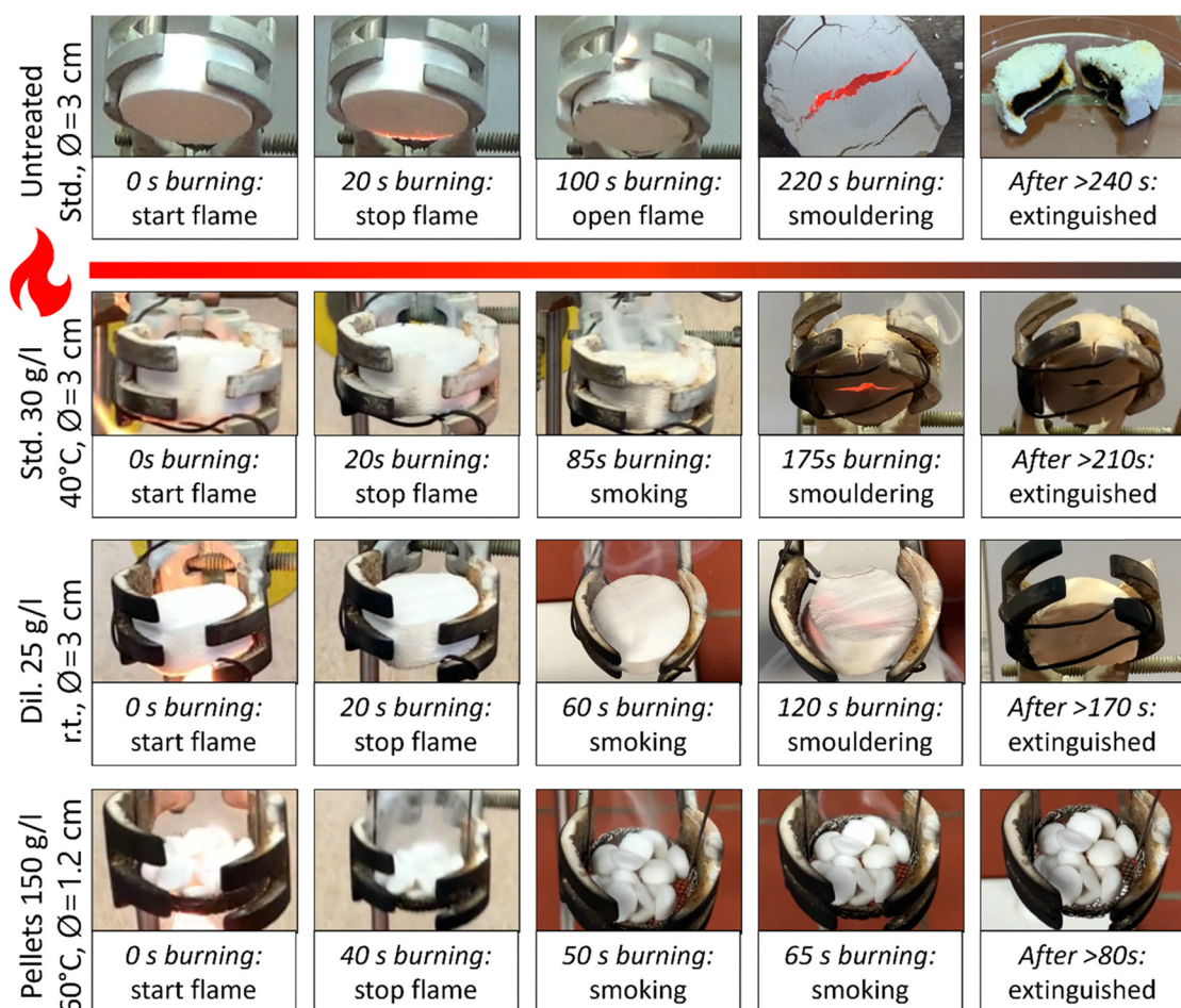
Fig. 4 Detailed progression of selected burn experiments at different times.
