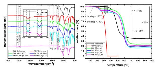
Fig. 2 Stacked IR-spectra (I.) and TGA data (r., under N2) of selected TPP-treated aerogel samples.
