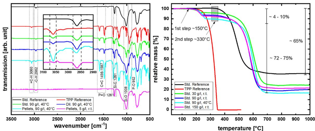
**Fig. 2** Stacked IR-spectra (l) and TGA data (r, under N<sub>2</sub>) of selected TPP-treated aerogel samples.
