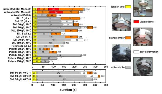
Fig. 3 Burn durations (top I.) and stages (r.) of untreated and selected TPP-treated aerogel samples and the reproducibility of the experiment (bottom I.).
