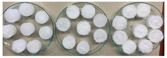
Fig. 1 Growth of TPP excess crystals during evaporation at r.t., with increasing concentration from left to right. These were removed before doing any calculations or experiments
