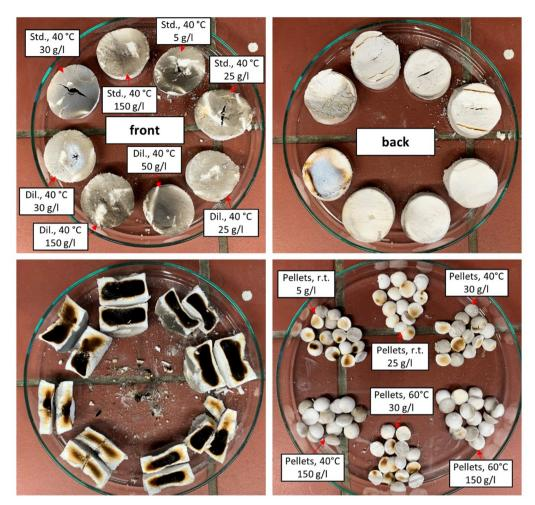
Sample pictures after the burn experiments: side exposed to the flame (top l.); backside (top r.); cross section (bottom l.); pellets (bottom r.).
