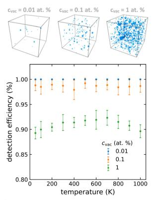
**Fig. 7** Vacancy detection validation. Top: Microstructures with varying void volume fractions are analysed for monovacancies and divacancies as a function of temperature. Bottom: The fraction of detected over nominal vacancies, the detection efficiency, is found to be insensitive to thermal noise.
