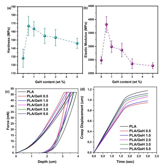
Fig. 6 Comparison of the (a) hardness; (b) elastic moduli; (c) typical load-depth nanoindentation curves and (d) representative creep displacement–time curves for neat PLA and PLA/GeH with various concentrations of the nanofiller.
