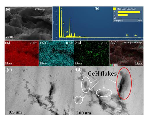
Fig. 3 SEM, EDS mapping and TEM images of the PLA/GeH 5.0 bulk: (a) SEM image obtained in the cross section of the film; (b) EDS spectra and elemental mapping  $(a_i)$ – $(a_{ii})$  along with the combined EDS layered image  $(a_{iv})$ ; (c) and (d) TEM images of the PLA/GeH 5.0.
