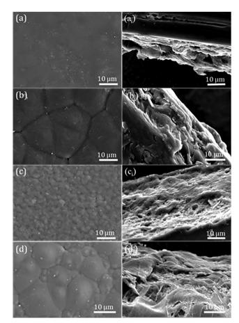
Fig. 2 SEM images of the surface (left) and the cross section (right) of bulk samples of (a) and (ai) neat PLA; (b) and (bi) PLA/GeH0.5; (c) and (ci) PLA/ GeH2.0 and (d) and (di) PLA/GeH5.0
