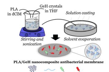
Scheme 1 Schematic representation of the experimental procedures followed for the fabrication of the PLA/GeH nanocomposites and the evaluation of the bactericidal properties.
