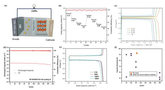
Fig. 6 (a) Schematic configuration of NF-NiO450@Li∥LiFePO<sub>4</sub>. Rate performance (b) and (c) and long-cycle performance (d)-(e) of the NF-NiO450 anode-assembled full cell with the LiFePO<sub>4</sub> cathode. (f) Comparison of capacity retention rates of partial 3D current collectors used in LMBs.
