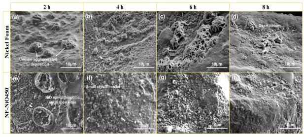
Fig. 5 Top-view SEM images of various anodes with lithium deposition of (a) and (e) 2 mAh cm<sup>-2</sup>; (b) and (f) 4 mAh cm<sup>-2</sup>; (c) and (q) 6 mAh cm<sup>-2</sup> and (d) and (h)  $8~\text{mAh}~\text{cm}^{-2}$
