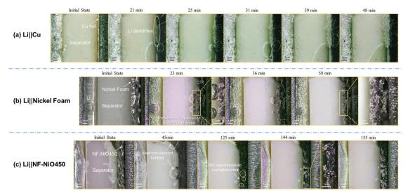
Fig. 4 The deposition morphology of metallic lithium on the current collector in in situ cells observed under an in situ polarized light microscope: (a)  $Li \parallel Cu$ , (b)  $Li \parallel NF$ , and (c)  $Li \parallel NF$ -NiO450
