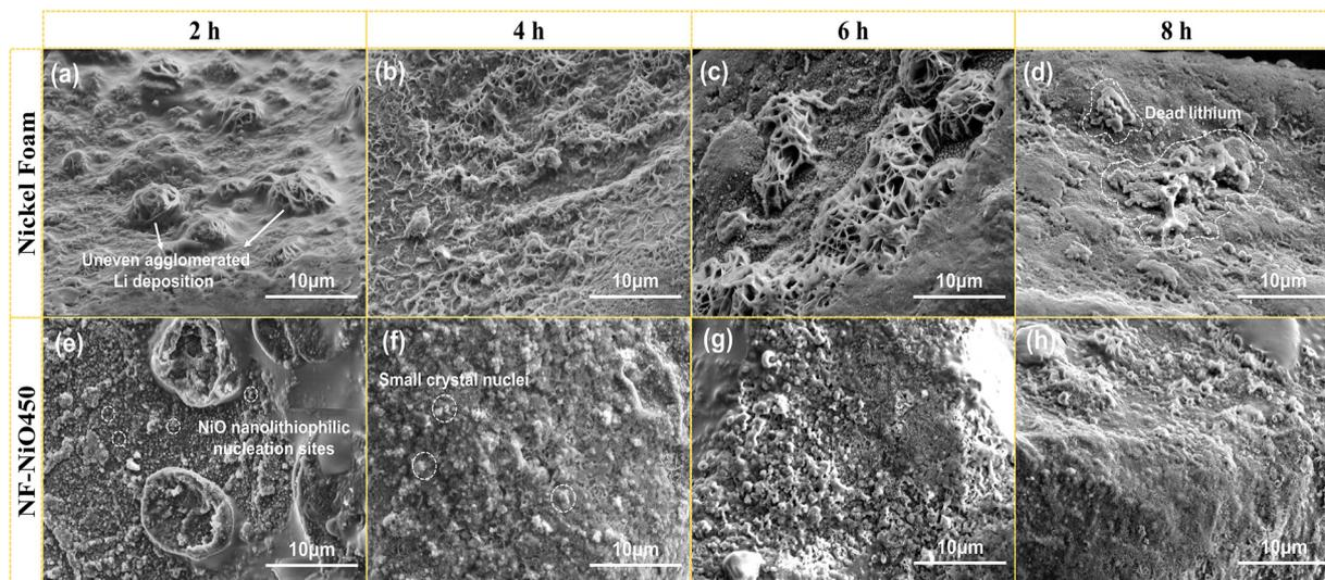
Fig. 5 Top-view SEM images of various anodes with lithium deposition of (a) and (e)  $2 \text{ mA h cm}^{-2}$ ; (b) and (f)  $4 \text{ mA h cm}^{-2}$ ; (c) and (g)  $6 \text{ mA h cm}^{-2}$  and (d) and (h)  $8 \text{ mA h cm}^{-2}$ .
