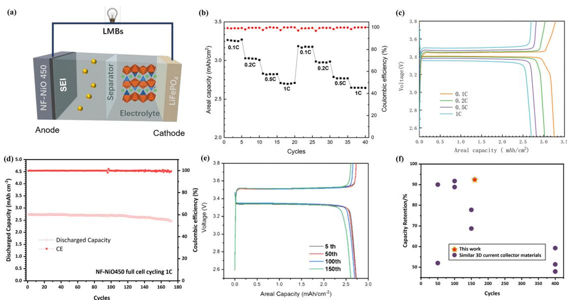
Fig. 6 (a) Schematic configuration of NF-NiO450@Li||LiFePO<sub>4</sub>. Rate performance (b) and (c) and long-cycle performance (d)–(e) of the NF-NiO450 anode-assembled full cell with the LiFePO<sub>4</sub> cathode. (f) Comparison of capacity retention rates of partial 3D current collector materials used in LMBs.
